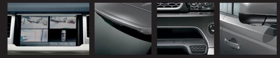
Five digital cameras are housed around the vehicle; two on either side of the front bumper, one in each of the door mirror casings and one in the rear spoiler.
