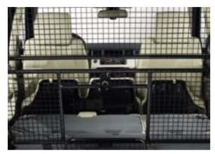
Cargo Barrier\* VUB502080 Easily removed, incorporates useful integral ski hatch.
