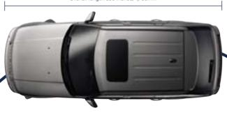
Turning Circle Curb-to-curb 37.7ft/11.5m Wall-to-wall 39.0ft/11.9m Turns lock-to-lock 3.1
