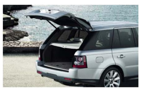
The power tailgate adds practicality and makes life with your Range Rover Sport even easier. Opened at the touch of a button on either the fascia or key fob, the opening height is programmable to suit personal preferences and accommodate more confined loading areas. The tailgate is closed via a button on the inside of the trunk lid.
