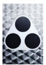
Tracking Target Sticker LR021589 Additional sticker required for vehicles equipped with Surround Camera System option which includes Tow Assist.
