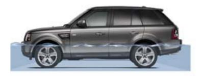
Wading Depth Maximum wading depth 27.5 inches/700mm
