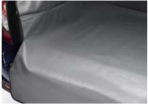
Flexible Loadspace Protector VPLSS0016 Heavy duty fabric protects loadspace up to window height. Covers full loadspace even with rear seats folded. Includes protective gloves.
