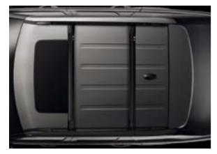
Roof Rails and Crossbars\* VUBS02130 Crossbars easily removed when not in use. Vehicle height when fitted 73.74 inches at normal ride height. Maximum payload 158.29lbs†.
