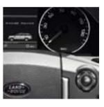
Easy-to-use Human-Machine-Interface (HMI) Touch Screen with entertainment, information, navigation and communication functionality.
