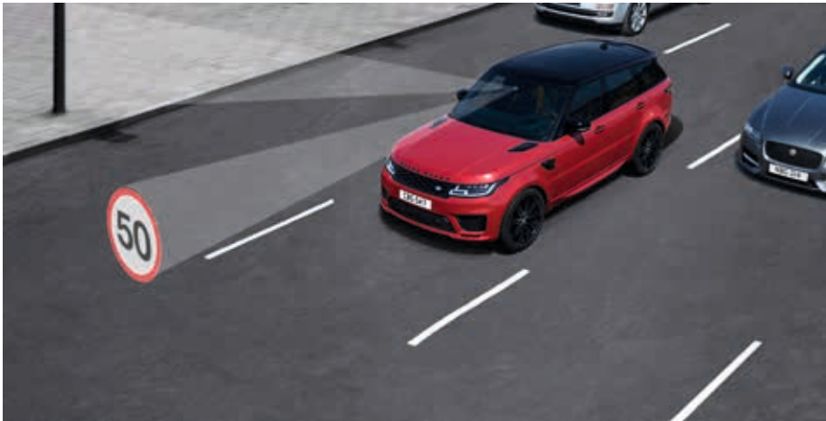
Traffic Sign Recognition with Adaptive Speed Limiter
