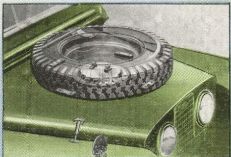
Alternative position for carrying the spare wheel ; a special fitting can be supplied.
