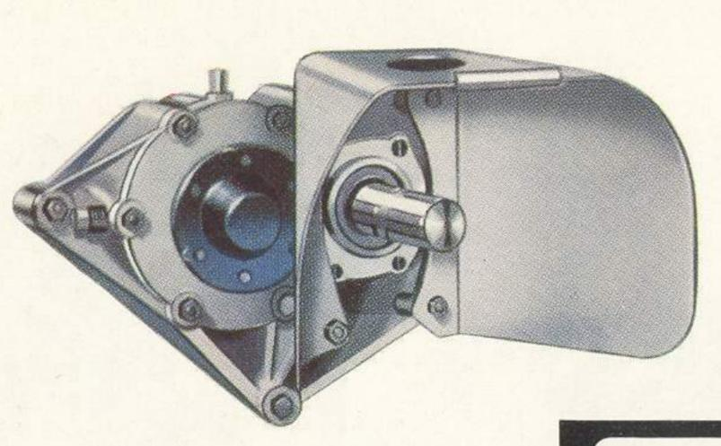
Rear power take-off drive section for operating, through a splined shaft, machinery towed by the vehicle.
