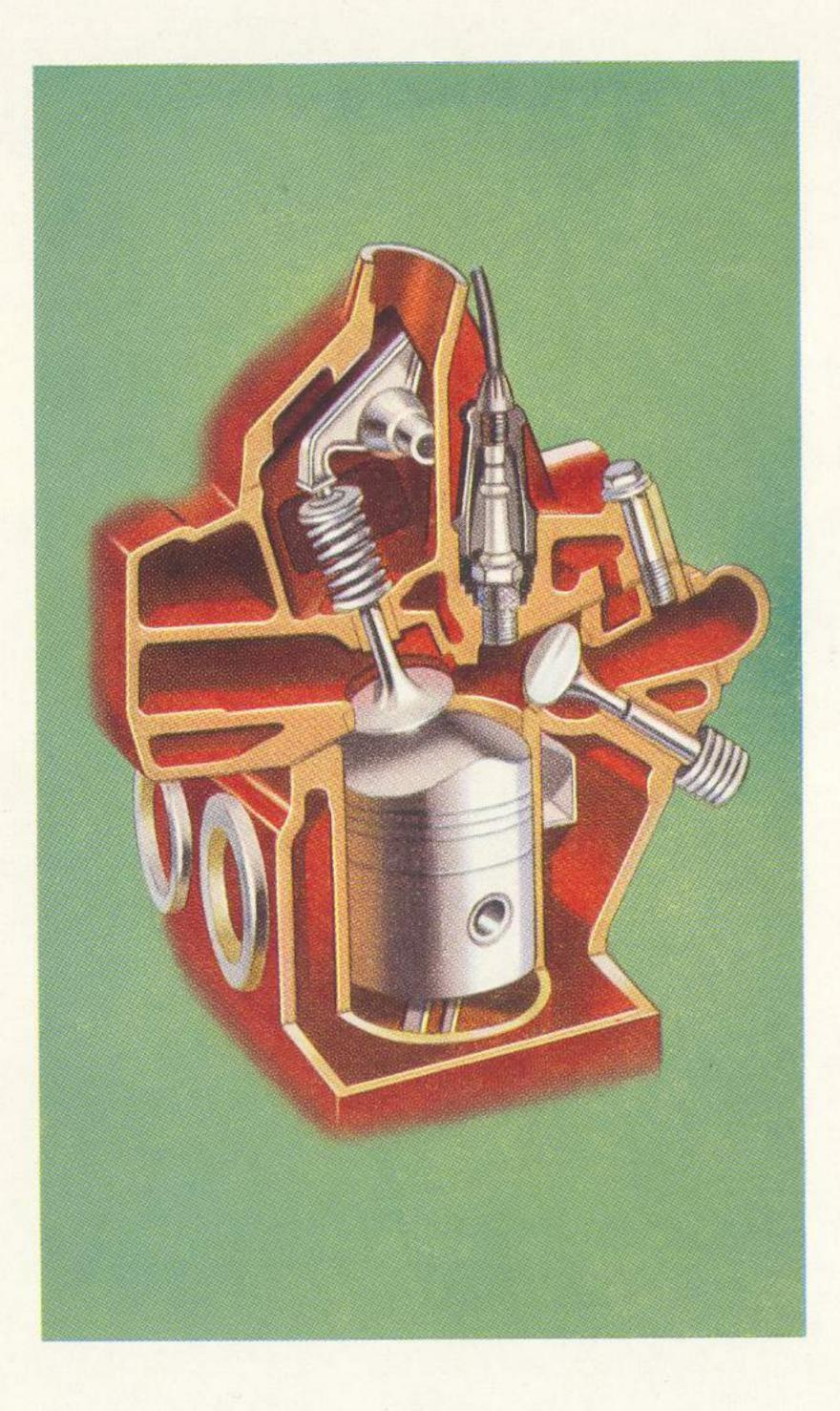
Power for vehicle operation, power for hauling trailers, power for driving machinery. Power that is smooth and willing for normal work ; slogging determined power for the tough jobs. The overhead inlet and side exhaust valve design of the Land-Rover engine ensures that all this power is developed with maximum efficiency and economy. It is a reliable unit, its robust construction giving it a long, trouble-free service life.
