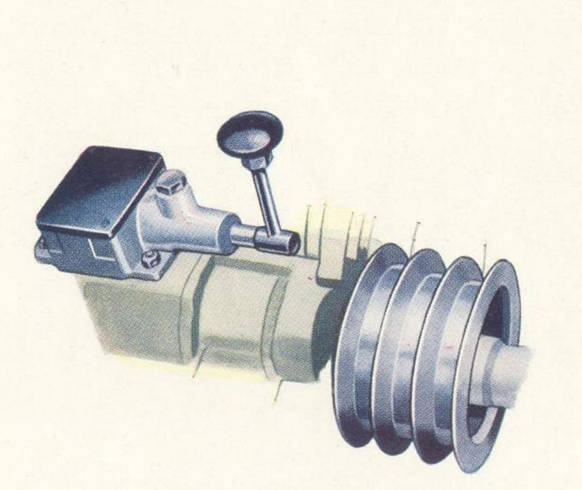
Centre power take-off may be used to operate an appliance mounted in the body of the vehicle.
