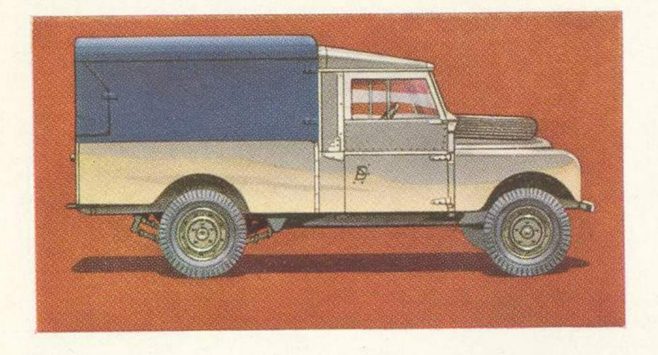
For difficult cross-country work loads of 1,200 lb. (544 kg.) can be carried in addition to the driver and two passengers, while on journeys using more normal road surfaces, payloads of 1,500 lb. (680 kg.) can be satisfactorily dealt with.
