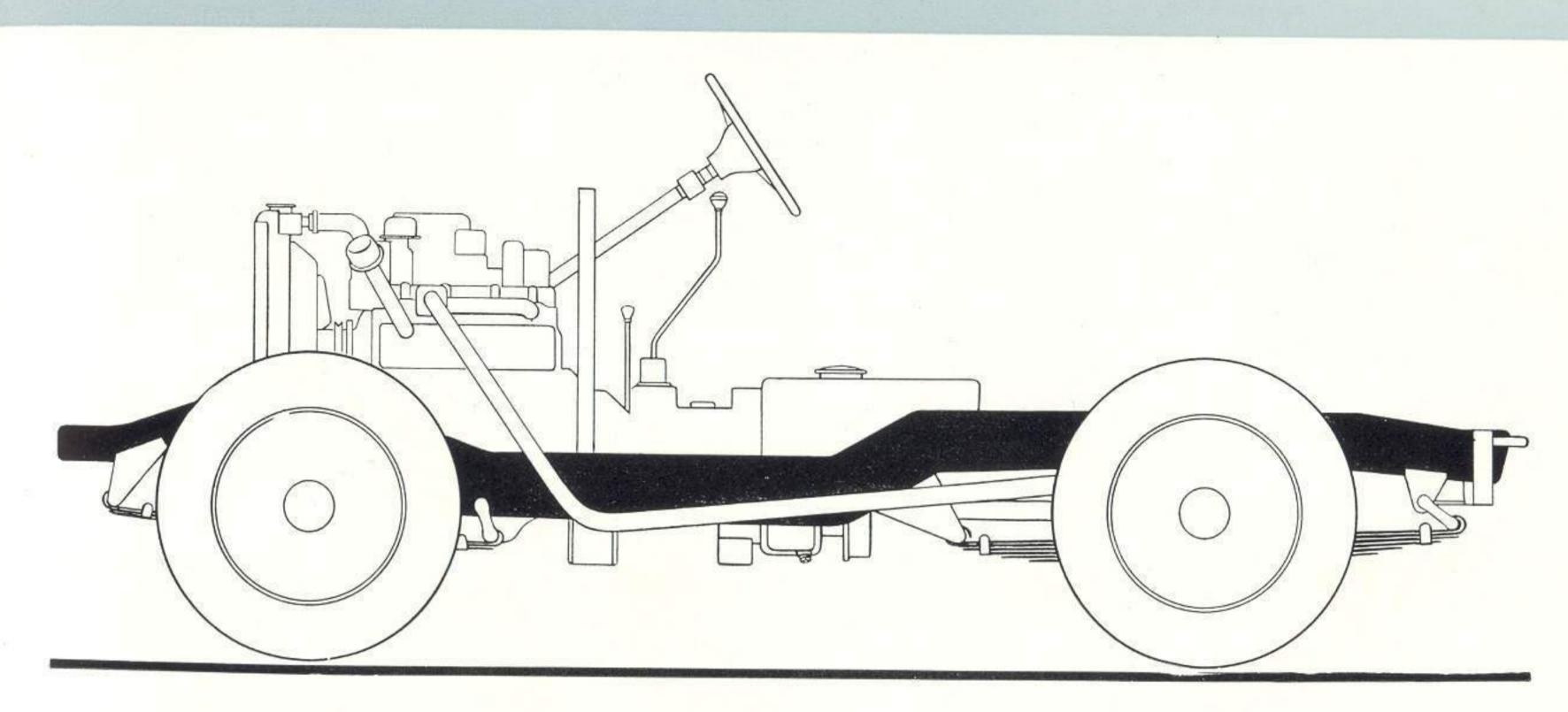
Air Cleaner and Silencer : A.C. large capacity oil bath type, with built-in pre-cleaner.
