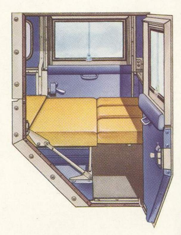
Additional seats mounted on the rear wheel boxes will carry four passengers, two on each side.
