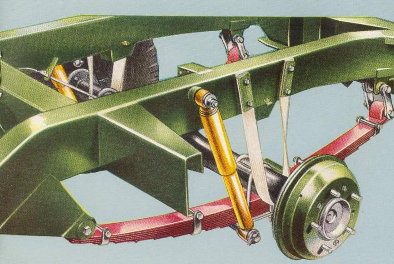
Land-Rover brakes are hydraulically operated. Leading and trailing shoes are used for 86 in. wheelbase models, while 107 in. wheelbase vehicles employ two-leading shoes on front wheels.
