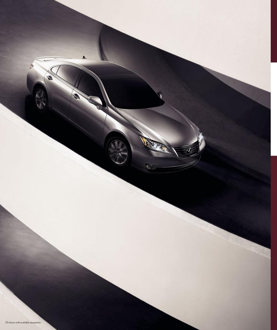
An available Dual-swivel Adaptive Front Lighting System (AFS)<sup>6</sup> can help illuminate curves by rotating the right or left headlamp up to 15 degrees into a turn at speeds below 19 mph and both headlamps together at speeds above 19 mph.
