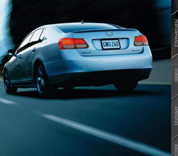
While the GS 460 can go from 0 to 60 in 5.4 seconds, what's truly extraordinary is how seamlessly it gets you there. An eight-speed sequential-shift automatic transmission glides through its gears, while Variable Valve Timing with intelligence and Electronic intake valve timing (VVT-iE) continuously adjusts the timing of the engine's valves to deliver optimum performance at all times. It's like starring in your own action movie—in perpetual fast-forward.
