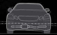
The available Active Stabilizer Suspension System uses sensors and actuators to help reduce body tilt while cornering.
