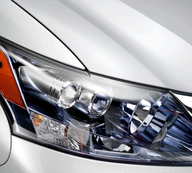
The best way to improve vision is to outthink what impairs it. Enter the available LED Dual-swivel headlamps with Adaptive Front Lighting System (AFS). It enables the LED headlamps to turn so they're better able to illuminate curves. They're even capable of independent thought. At speeds above 19 mph, both headlamps swivel into a curve, illuminating more of the road ahead. At lower speeds, the left headlamp rotates up to 15 degrees while the right headlamp rotates up to 10 degrees.
