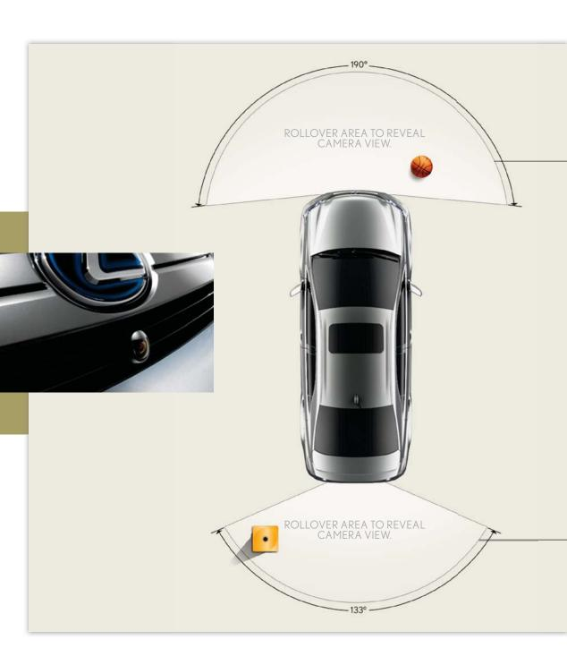
Using a specially designed wide-angle lens to help reveal hard-to-see areas, an available Wide-view Front Monitor<sup>5</sup> comes on at the touch of a button (or automatically, if you choose) when you're driving at low speeds. A camera mounted in the grille displays a 190-degree front view on the navigation screen.
