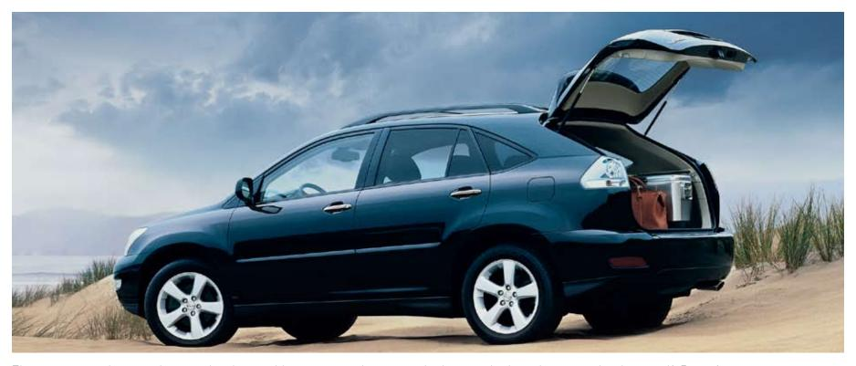
The power rear door can be raised or lowered by pressing a button on the key, inside the cabin or on the door itself. For safety purposes, a series of beeps will alert those standing nearby whenever the door function is activated. If the button is activated while cargo is being loaded, a resistance sensor will prevent the door from lowering.
