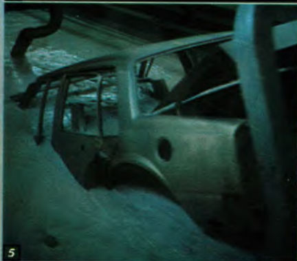
1. Computers aid in design and manufacture. 2. Worker team. 3. Robotic spray booth. 4. Instrument panel checking station. 5. ELPO bath of rust-resistant primers. 6. Robogate body framing. 7. Final computerized process check.
