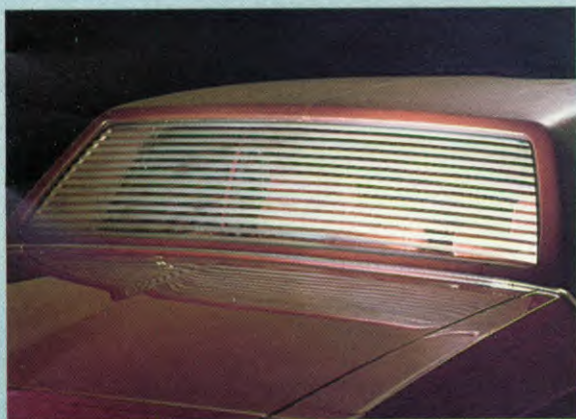
Rear window defogger. Electric filaments in the glass defog the window quickly and silently.
