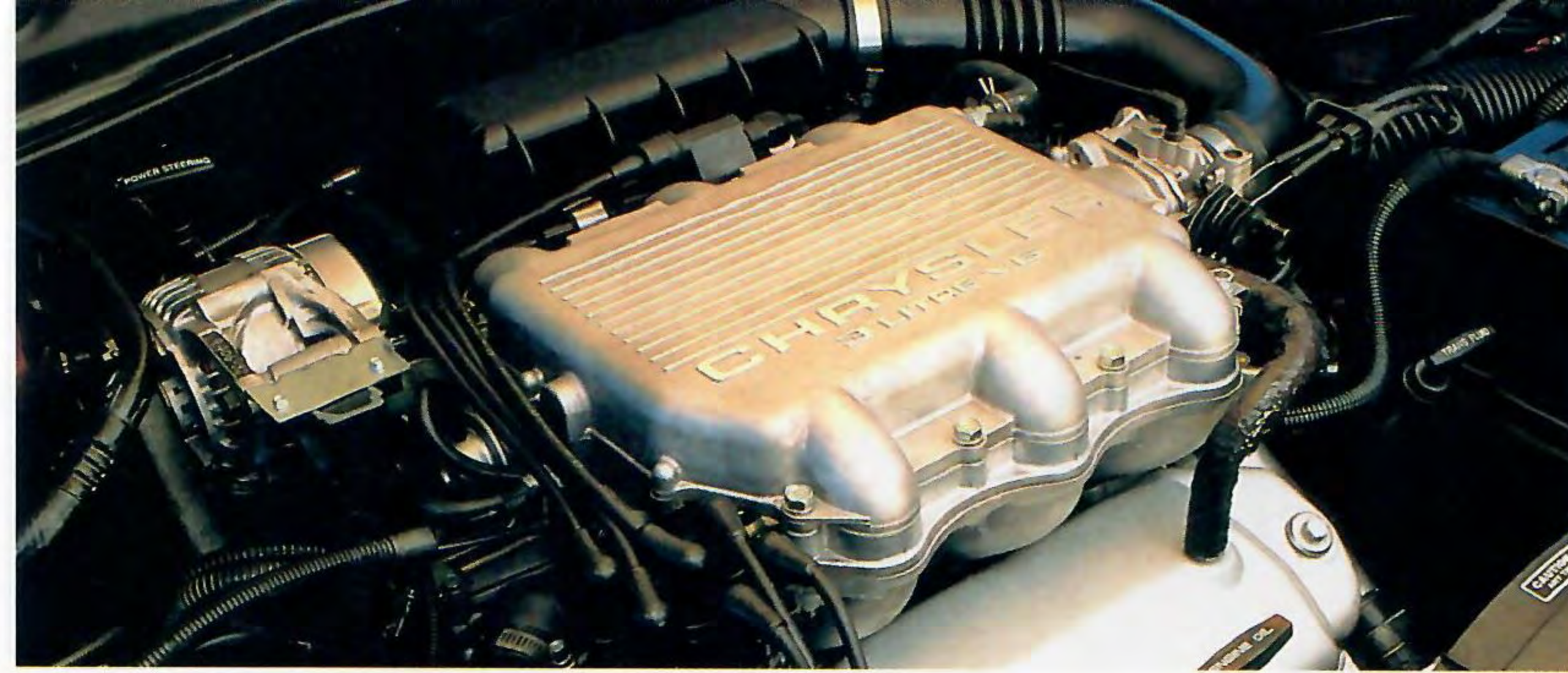
Acclaim's available 3.0-liter V6 engine now has SMPI (sequential multipoint fuel injection) for efficiency and easy cold-weather starting. A 2.5-liter EFI (electronic fuel injection) engine is standard.
