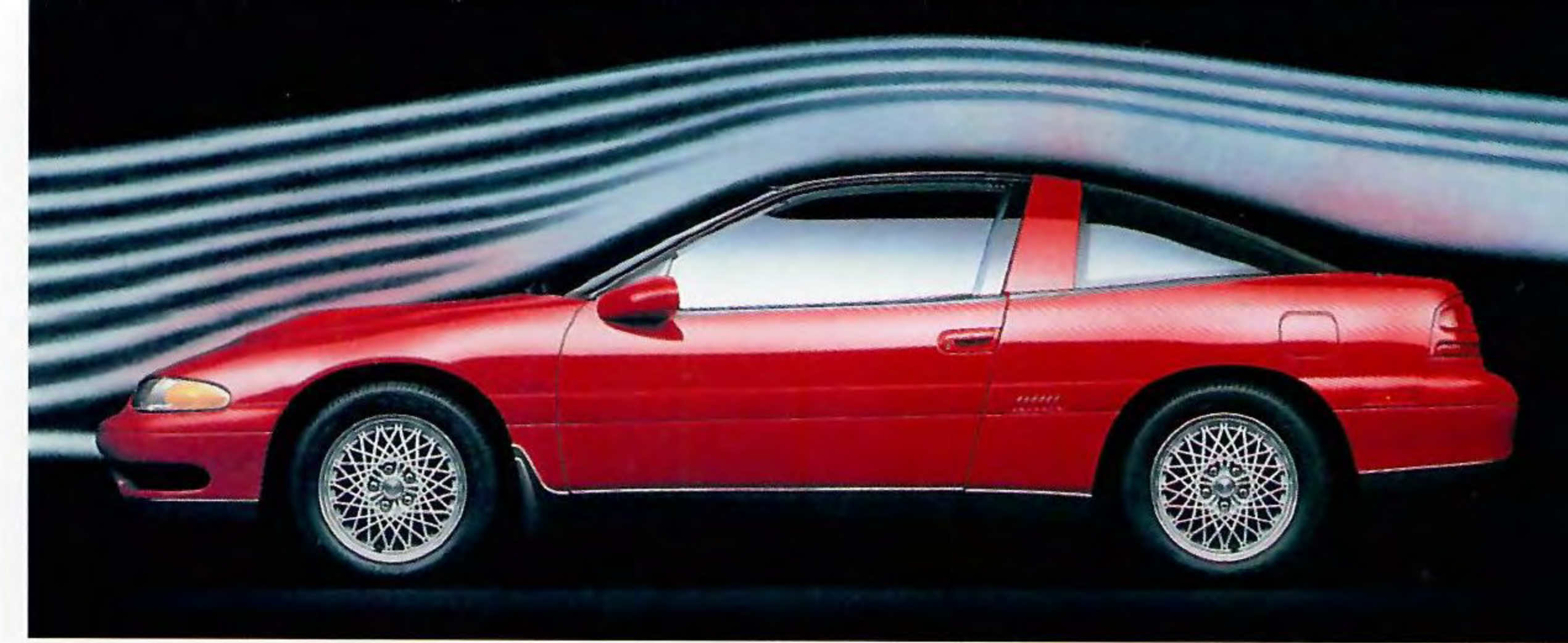
Laser's contemporary and aerodynamic shape has earned an impressive drag coefficient of 0.33. A new rear spoiler (available February 1992) is standard on Laser RS Turbo and RS Turbo AWD models.
