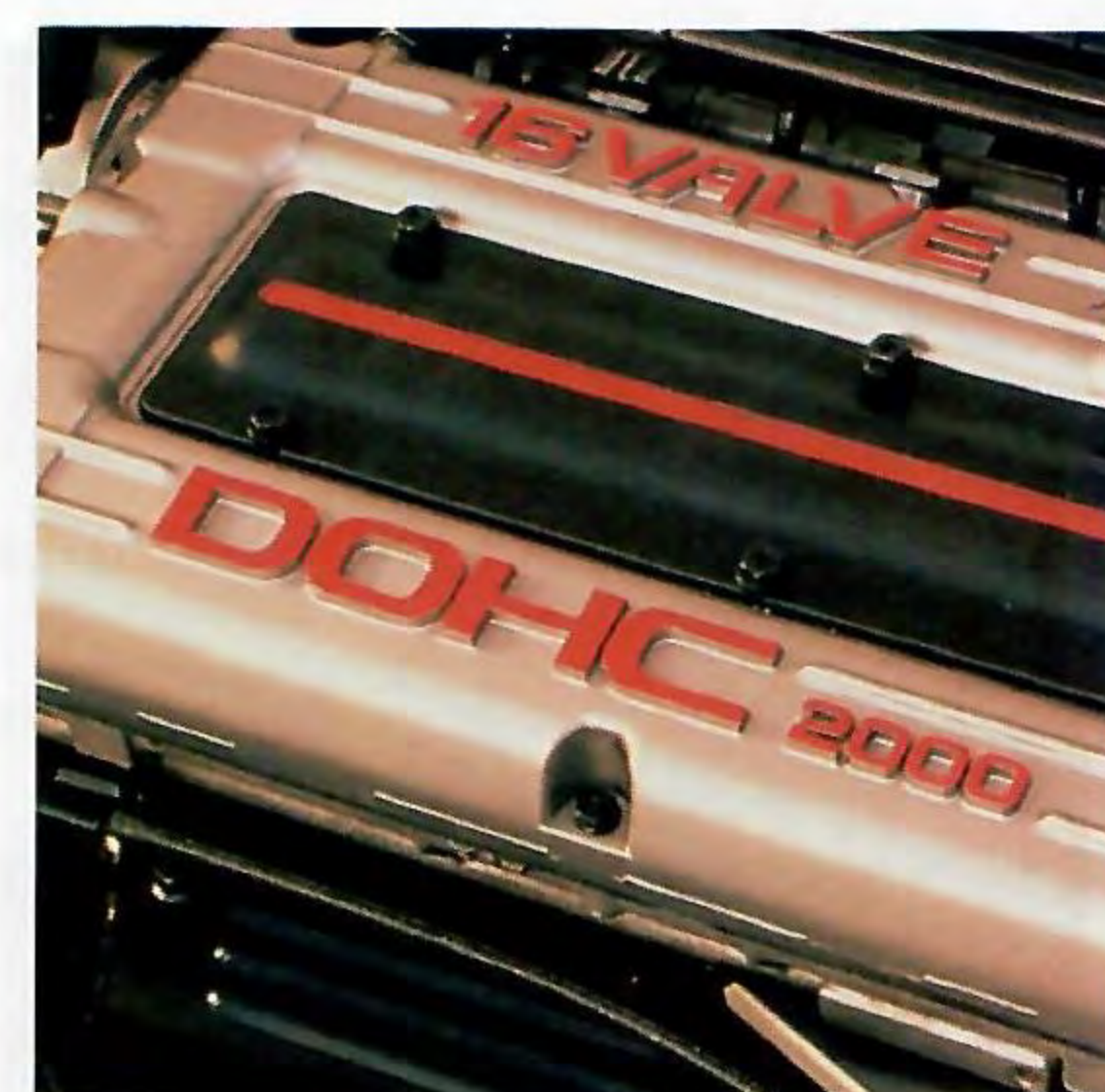
2.0-liter DOHC 16-valve intercooled turbocharged MPI engine delivers 195 horsepower with five-speed manual transaxle.
