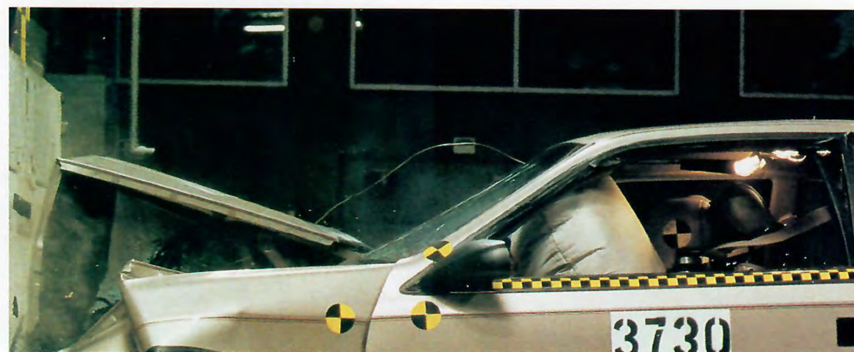
Crash characteristics of vehicle body and chassis components are accurately measured through extensive collision testing. Computer simulation is another process for achieving the goal of maximum driver and passenger safety.
