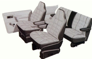
Voyager. Standard deluxe cloth with vinyl trim reclining high-back front bucket seats with integral head restraints, inboard folding armrests, and passenger seatback assist handle. Includes a three-passenger rear bench seat in matching trim. Seven-passenger seating is optional on Voyager. In Almond, Bordeaux, Silver/Charcoal.
