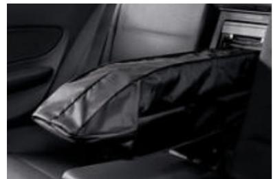
**Ski bag** allows clean and secure transport of four pairs of skis and ski poles as well as other long items. When the ski bag is not extended, it can be stored out of sight to save space, and the fold-down center armrest can be left down for use.
