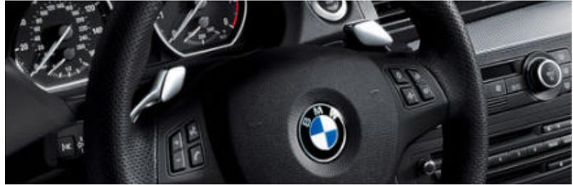
□ **Steering wheel-mounted paddle shifters** allow you to shift gears manually without a clutch. This optional feature comes included in the 1 Series Coupe when it is equipped with optional STEPTRONIC automatic transmission and Sport Package.
