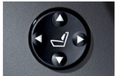
**Lumbar support** for front seats adds four-way power-adjustable comfort for the lower back. Lumbar support can be adjusted up/down and in/out.
