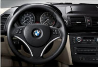
■ **Three-spoke leather-wrapped multi-function steering wheel** lets you keep both hands on the wheel while adjusting various comfort functions, such as controls for audio system, cruise control and hands-free phone controls.
