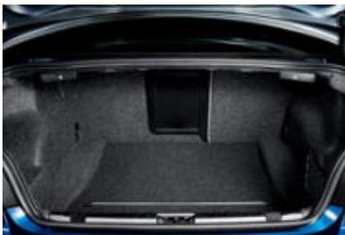
■ **Lined luggage compartment** is illuminated and can be expanded by folding down the split-folding rear seats. An elastic strap on the left-hand side, a flexible storage net on the right and lashing points on the inside edge help to ensure safe transportation of cargo. (Shown with optional Cold Weather Package pass-through opening for ski bag.)
