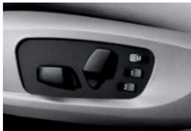
**Power seat adjustments** included with 8-way power front seats allow customized comfort and convenience for driver and front passenger. The two-setting memory system automatically adjusts the driver's seat and side-view mirror positions so individual preferences are always available at the touch of a button.
