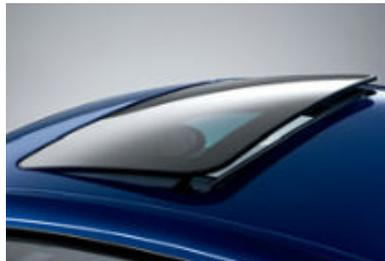
■ **Two-way power glass moonroof** with remote, expanded one-touch operation, slides backward or tilts up to let in as much fresh air and sky as you like, while a wind deflector helps keep the wind out. Includes a sliding interior sunshade.
