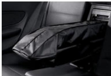
□ **Ski bag**, included in the Cold Weather Package, allows clean and secure transport of four pairs of skis and ski poles as well as other long items. When the ski bag is not extended, it can be stored out of sight to save space, and the fold-down center armrest can be left down for use.
