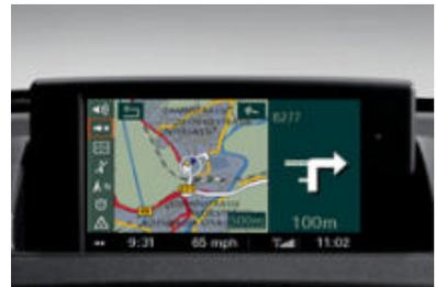
□ **Navigation system** covers the U.S. with a single DVD. The glare-free monitor is mounted neatly into the dashboard for easy viewing. Using GPS satellites and DVD technology, a map of your area appears on the dash monitor, showing – and telling – the directions to your desired destination. It also provides Real Time Traffic Information on potential traffic problems and solutions.
