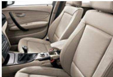
■ **Standard front seats**, shown here with optional Taupe Boston Leather upholstery and iDrive, offer 8-way manual adjustment including 2-way adjustment of headrests. The front passenger seat also includes manual height adjustment.
