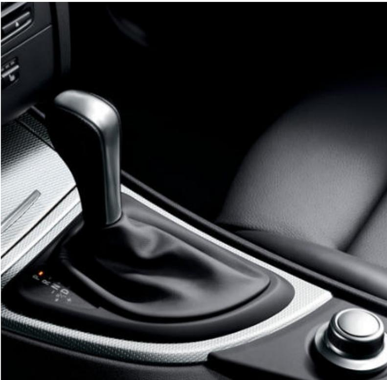
□ **6-speed STEPTRONIC automatic transmission** provides a choice of three modes: “Drive,” which incorporates BMW’s Adaptive Transmission Control; “Sport” automatic, for a more dynamic shift pattern; and STEPTRONIC automatic, for the hands-on control of a manual without using a clutch.
