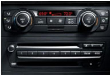
■ **Automatic climate control system** allows occupants to select a specific cabin temperature and choice of fan speeds, as well as automatic or manual airflow and recirculation. The automatic recirculation control activates whenever certain air pollutants are detected. The system also includes defrost/demist and MAX A/C functions.
