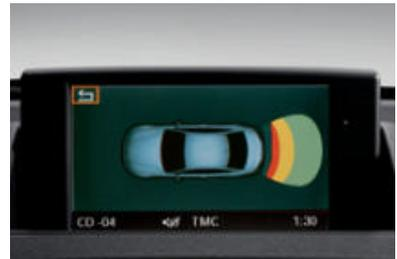
□ **Park Distance Control** uses ultrasonic sensors in the rear bumper to help you judge the distance to other cars and unseen objects when parking. The beeping becomes faster as your bumper approaches the object, turning into a constant tone when the distance is less than 12 inches.
