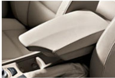
■ **Front armrest** with integrated storage compartment folds up to allow access to the front cupholder(s), shown at left, and Auxiliary input port shown on page 53.
