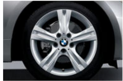
**Star Spoke (Style 262) light alloy wheels and run-flat<sup>2</sup> performance tires.<sup>3</sup>** In front: 17 x 7.0 wheels and 205/50 tires; in back: 17 x 7.5 wheels and 225/45 tires.<sup>3</sup> (included in 128i Sport Package)
