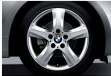
□ Star Spoke (Style 142) light alloy wheels with run-flat<sup>1</sup> all-season tires. In front: 17 x 7.0 wheels and 205/50 tires; in back: 17 x 7.5 wheels and 225/45 tires.<sup>3</sup> (No-cost opt. on 135i)
