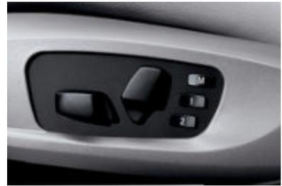
□ **Power seat adjustments** included with 8-way power front seats allow customized comfort and convenience for driver and front passenger. The two-setting memory system automatically adjusts the driver's seat and side-view mirror positions, with individual preferences available at your fingertips.
