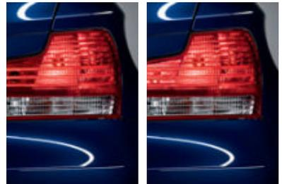
■ **Adaptive Brake Lights** increase vehicle visibility and signal the intensity of your braking action. In the event of an emergency stop, the illuminated area of the brake lights is increased, so traffic following behind you knows to stop quickly.
