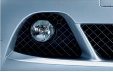
■ **Halogen free-form foglights** are cleanly integrated into the front bumper, illuminating the road ahead in bad weather.
