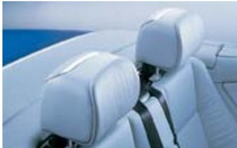
■ **Rear headrests** help protect the heads and necks of rear-seat occupants in an impact or sudden stop. BMW’s Rollover Protection System bars are discreetly integrated for additional safety, in case of rollover.
