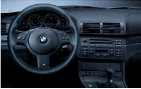
**M three-spoke leather-wrapped multi-function sport steering wheel** has fingertip cruise, audio and telephone<sup>1</sup> controls.
