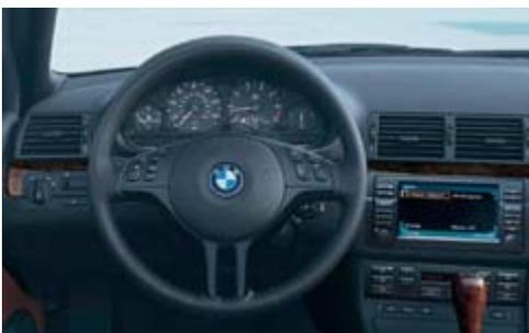
■ A **three-spoke leather-wrapped multi-function sport steering wheel** lets you keep both hands on the wheel while adjusting audio settings, cruise control and using the accessory phone. (Optional navigation system shown.)
