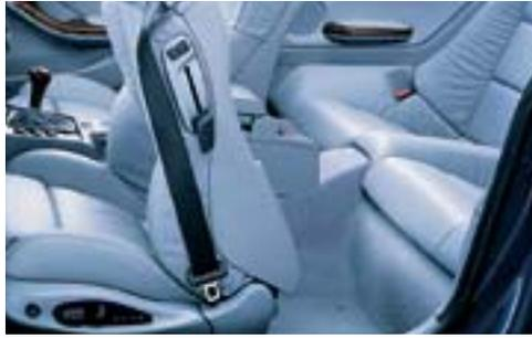
■ Ingenious **seatback easy-entry feature** offers power fore/aft controls that may be used to move the seat forward all the way for easy access, then back again to the seat’s original position. Each front seat has two sets of fore/aft controls – the controls on top move the seat double-speed, for quickest access.
