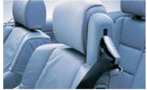
■ **Seat-integrated front safety belts** help keep occupants firmly and comfortably in place. The seat-integrated design also helps ease entry and exit for rear-seat passengers.
