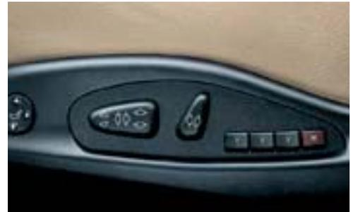
■ **Power front seats** include a **driver’s seat and mirror memory system**, which lets up to three drivers set their preferred seat and exterior mirror positions. (Plus, the passenger’s-side mirror tilts down when vehicle is shifted into reverse gear.) (Lumbar support shown standard in 330Ci; included in 325Ci Premium Package.)
