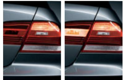
■ **Adaptive Brake Lights** help other drivers recognize the intensity of your braking actions. In emergency braking, the illuminated area of the brake lights increases, alerting drivers behind you to brake quickly.
