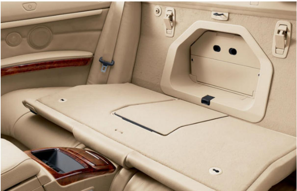
**Through-loading hatch** opening is almost 16 inches wide. With the backrest folded down, skis, snowboards, and other long items can be transported – even with the top down. Two fastener hooks conveniently transport items, such as grocery bags, in an upright position.
