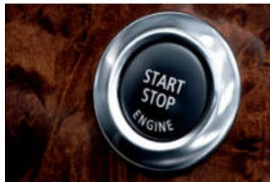
■ **Engine Start/Stop button**<sup>4</sup> and remote key control the engine. First, insert the remote key into the starter switch slot. After the electronic identification system confirms that it is the correct remote key, you can start (or later, turn off) the engine by pressing the Start/Stop button.
