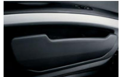
■ **Storage compartments** are integrated into both doors. A tilt-out bin below the armrest offers different compartments in which to tuck away sunglasses, change and other small items; a convenient open storage space for maps and larger items is just behind it.
