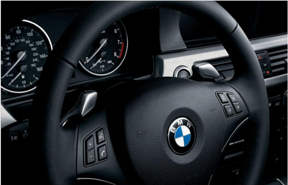
□ **Steering wheel-mounted paddle shifters**<sup>1</sup> allow you to quickly upshift and downshift without a clutch.
