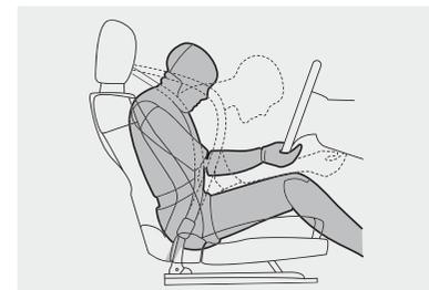
**BMW restraint system** for the driver and front passenger combines three-point safety belts, automatic safety-belt pretensioners, seat bolsters that help prevent occupants from sliding forward, and head restraints. This system helps provide optimum restraint in a collision.
