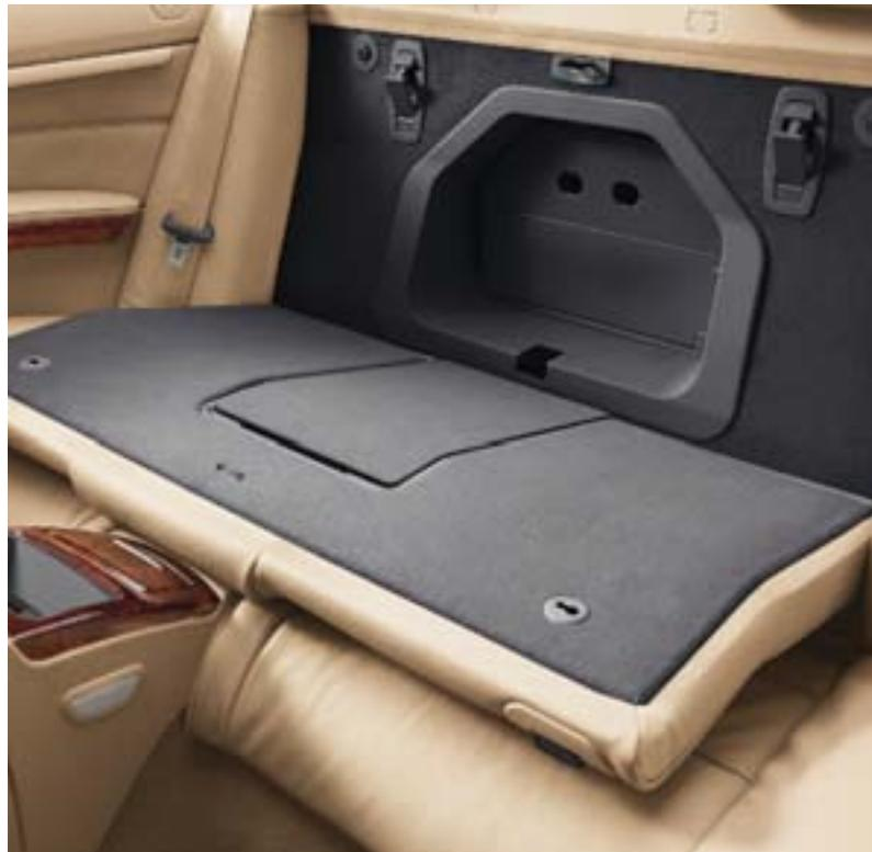
**Through-loading hatch** opening is almost 16 inches wide. With the backrest folded down, skis, snowboards, and other long items can be transported even with the top down. Two fastener hooks conveniently transport items, such as grocery bags, in an upright position.
