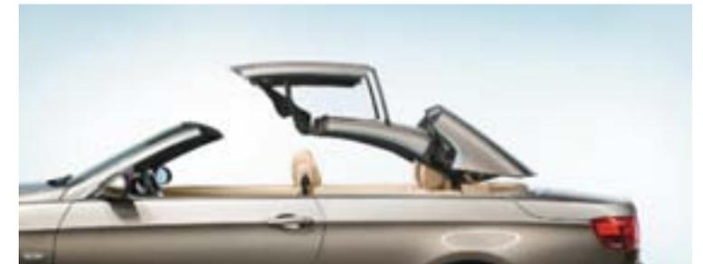
**3. The three parts of the roof smoothly move towards the rear and stack, one above the other, while the trunk lid unlocks at the front and swings up.**
