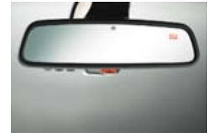
**BMW Universal garage-door opener** takes the place of up to three remote-control devices, helping to eliminate clutter. It can activate remote functions outside the vehicle, such as garage-door openers or home-lighting systems. Also shown: the **automatic-dimming rear-view mirror** with digital compass.
