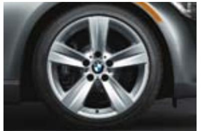
**Star Spoke (Style 189)** light alloy wheels with **run-flat<sup>1</sup> performance tires.<sup>2</sup>** In front: 18 x 8.0 wheels with 225/40 tires; in back: 18 x 8.5 wheels with 255/35 tires. (335i Sport Package)
