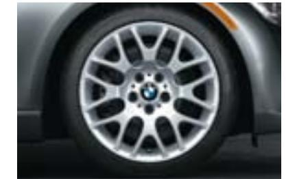
□ **Cross Spoke (Style 197)** light alloy wheels with run-flat<sup>1</sup> performance tires.<sup>2</sup> In front: 18 x 8.0 wheels with 225/40 tires; in back: 18 x 8.5 wheels with 255/35 tires. (Included in 328i Sport Package.)
