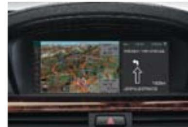
□ **Navigation system** features a high-resolution, glare-free monitor. Using GPS satellites in conjunction with data stored on an internal hard drive, a choice of detailed maps show and tell the directions to your desired destination. In many areas, it also provides Real Time Traffic Information on potential traffic problems along your route, and can even plan a detour around them.
