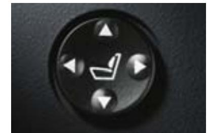
**Lumbar support** for front seats adds four-way adjustable comfort for the lower back. Lumbar support can be adjusted up/down and in/out.
