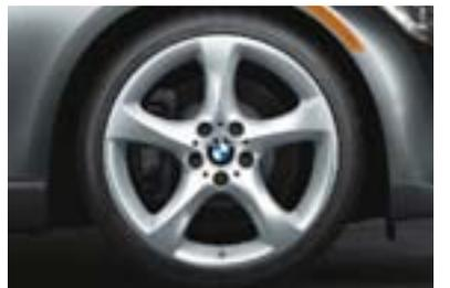
**Star Spoke (Style 230)** light alloy wheels with **run-flat<sup>1</sup> performance tires.<sup>2</sup>** In front: 19 x 8.0 wheels with 225/35 tires; in back: 19 x 9.0 wheels with 255/30 tires. (Optional on 335i, requires optional Sport Package.)
