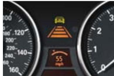
□ **Active Cruise Control** system uses radar measurements to automatically maintain a preset speed and distance between your vehicle and the one ahead in highway driving.<sup>1</sup>
