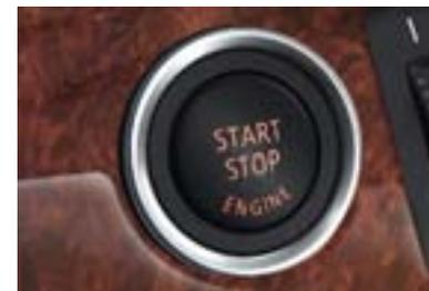
■ **Engine Start/Stop button<sup>3</sup> and remote key** control the engine. First, insert the remote key into the starter switch slot. After the electronic identification system confirms that it is the correct remote key, you can start (or later, turn off) the engine by pressing the Start/Stop button.
