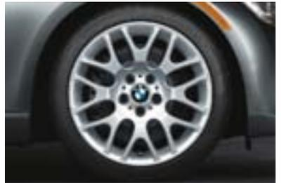
**Cross Spoke (Style 197)** light alloy wheels with **run-flat<sup>1</sup> performance tires.<sup>2</sup>** In front: 18 x 8.0 wheels with 225/40 tires; in back: 18 x 8.5 wheels with 255/35 tires. (328i Sport Package)
