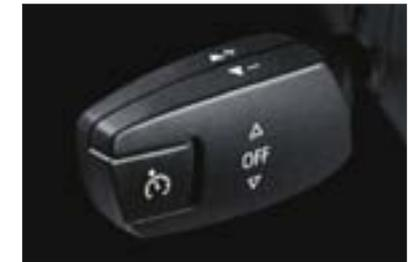
■ **Dynamic Cruise Control** lets you store and keep to a chosen speed above 20 mph, automatically applying the brakes on a downhill. It is activated via the left-hand steering column switch and deactivated by applying the brakes or via the switch.<sup>2</sup>
