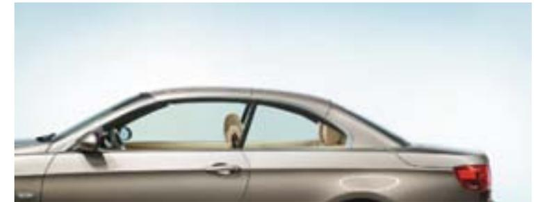
**2. With the vehicle stopped, holding down a button on the console or on the key fob, with Comfort Opening and Loading operates the motor that electrohydraulically unlocks and separates the three-part roof. As a safety measure, once the button is released, the motion stops.**
