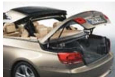
□ **Comfort Opening and Loading** feature (included with Comfort Access) offers a quick, easy way to stow and remove luggage or large packages from the trunk when the top is down. Simply press a button on the remote key to raise the hardtop up and out of the trunk and freeze it in position; another press neatly lowers the hardtop back into the trunk.
