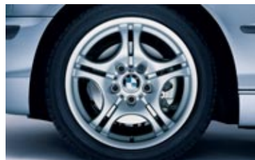
M Double Spoke (Styling 68M) alloy wheels and performance tires 1 complement the sport suspension to deliver breathtaking roadholding capabilities. In front: 17 x 7.5 wheels and 225/45R-17 tires; at the rear: 17 x 8.5 wheels and 245/40R-17 tires. (incl. with Optional 330i Sport Package)
