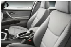
■ **Standard front seats**, shown here with optional Dakota Leather upholstery, offer eight-way manual adjustment, including two-way headrests with Active Headrests feature. The front passenger seat also includes manual height adjustment.
