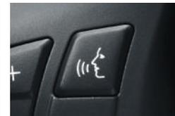
□ **Voice command** allows you to activate numerous Navigation system functions, record up to five minutes of notes, and dial hands-free. The Voice command button must be pressed before each use, so conversations won't accidentally activate the phone or other systems.
