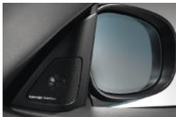
□ **Harman Kardon Surround Sound Audio System** with vehicle-specific equalizing and powerful 420W amplifier. The 13-speaker system includes four tweeters, four midrange speakers located in the door panels and two midrange speakers located under the rear shelf space, two bass speakers located under the front seats and one midrange center channel speaker located in the dashboard.
