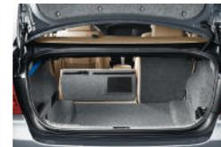
■ **Lined trunk** is illuminated and can be expanded by folding down either side of the optional split-folding 60/40 rear seats – or both at once to facilitate the transport of long items.
