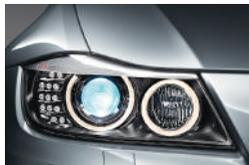
■ □ **Xenon Adaptive Headlights** brilliantly illuminate the road ahead and to the side at night and in conditions with poor visibility, while helping to keep glare away from oncoming drivers. BMW Adaptive Headlights provide optimum road illumination around corners, thanks to an electromechanical system that directs the headlights into and around the bend as soon as the vehicle begins cornering.
