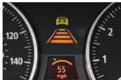
□ **Active Cruise Control** allows the driver to set a desired speed that is automatically maintained in free-flowing traffic. As a slower-moving vehicle is approached, a radar sensor alerts the system and adjusts speed to match the slower vehicle, while maintaining a preset following distance. As the lane ahead clears, the system automatically returns the car to the set speed.<sup>2</sup>
