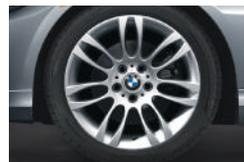
□ **Double Spoke (Style 195)** light alloy wheels and **run-flat<sup>1</sup> performance tires**.<sup>2</sup> In front: 18 x 8.0 wheels and 225/40 tires; in back: 18 x 8.5 wheels and 255/35 tires. (Included in 335d Sport Package.)
