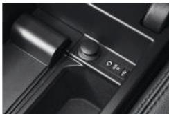
■ **Auxiliary input port** lets you connect an external audio source, such as an iPod® or MP3 player.
