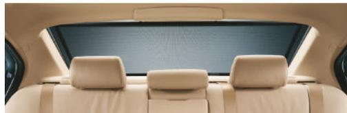
□ **Power sunshade for the rear window** can be raised and lowered at the press of a button. Together with manual sunshades for the rear side windows, this feature maintains occupant privacy, helps eliminate glare, and helps lower the cabin temperature by reflecting intense sunlight.
