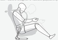
■ **BMW restraint system** for the driver and front passenger combines three-point safety belts, automatic safety-belt pretensioners, seat bolsters that help prevent occupants from sliding forward, and Active Headrests. This system helps provide optimum restraint in a collision.
