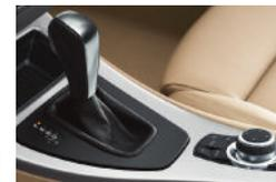
■ □ **6-speed STEPTRONIC automatic transmission** provides a choice of three modes: "Drive" with Adaptive Transmission Control; more dynamic "Sport" mode; and STEPTRONIC automatic, for the hands-on control of a manual without a clutch. (When ordered with the Sport Package or M Sport Package, steering wheel-mounted paddle shifters are automatically added.)
