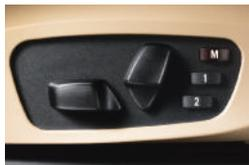
□ **Power seat adjustments** included with eight-way power front seats allow customized comfort and convenience for driver and front passenger. The two-setting memory system automatically adjusts the driver's seat and side-view mirror positions, with individual preferences available at your fingertips.
