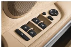
■ **Power window buttons** with "one-touch" up/down operation and **exterior mirror adjustment** controls are located conveniently to the left of the driver, allowing access that doesn't require taking your eyes off of the road.
