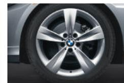
□ **Star Spoke (Style 287)** light alloy wheels and **run-flat<sup>1</sup> performance tires**.<sup>2</sup> In front: 18 x 8.0 wheels and 225/40 tires; in back: 18 x 8.5 wheels and 255/35 tires. (Included in 335i Sport Package; optional on 335i xDrive, requires optional Sport Package.)
