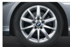
□ **Star Spoke (Style 286)** light alloy wheels and **run-flat<sup>1</sup> performance tires**.<sup>2</sup> In front: 17 x 8.0 wheels and 225/45 tires; in back: 17 x 8.5 wheels and 255/40 tires. (Included in 328i Sport Package; optional on 328i xDrive, requires optional Sport Package.)
