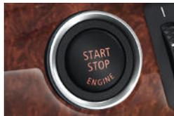
■ **Engine Start/Stop button<sup>1</sup>** and remote key control the engine. First, insert the remote key into the starter switch slot. After the electronic identification system confirms that it is the correct remote key, you can start (or later, turn off) the engine by pressing the Start/Stop button.
