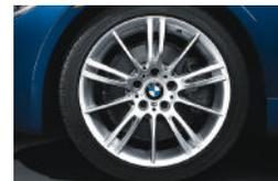
**Star Spoke (Style 193M)** M light alloy wheels and run-flat<sup>2</sup> performance tires.<sup>3</sup> In front: 18 x 8.0 wheels and 225/40 tires; in back: 18 x 8.5 wheels and 255/35 tires. (Included in 335i, 335i xDrive and 335d M Sport Package.)
