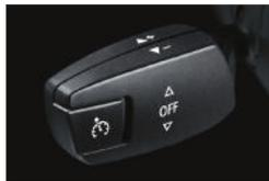
■ **Dynamic Cruise Control** lets you set and keep to a chosen speed above 20 mph, automatically applying the brakes downhill. It is activated via the left-hand steering column switch, and deactivated by applying the brakes or via the switch.<sup>2</sup>
