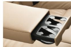
■ **Rear cupholders** are integrated into the front of the rear-seat center armrest. When not in use, they can be stored out of sight by sliding them back into the armrest.
