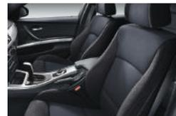
**Sport front seats** offer optimum lateral support during sporty driving maneuvers, and long-distance comfort when traveling. (Eight-way power front sport seats with two-way manual headrests and thigh support require Premium Package or power seats feature in 328i and 328i xDrive.)
