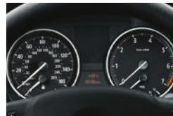
■ **Instrument panel** features a red backlight speedometer and tachometer. Centered between the two easy-to-read analog instruments is the on-board computer (at right) with liquid crystal display providing additional important driving information.
