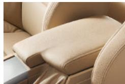
■ **Front armrest** with integrated storage compartment folds up to allow access to a front cupholder and Auxiliary input port shown on the facing page.
