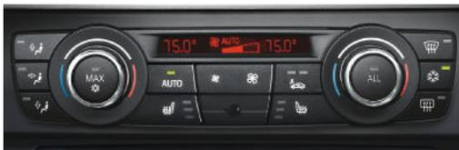
■ **Automatic climate control system** allows occupants to select a specific cabin temperature and choice of fan speeds, as well as automatic or manual airflow and recirculation. The automatic recirculation control activates whenever certain air pollutants are detected. The system also includes defrost/demist and MAX A/C functions.
