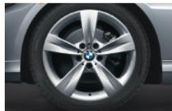
**Star Spoke (Style 287)** light alloy wheels and run-flat<sup>2</sup> performance tires.<sup>3</sup> In front: 18 x 8.0 wheels and 225/40 tires; in back: 18 x 8.5 wheels and 255/35 tires. (Included in 335i Sport Package; optional in 335i xDrive, requires optional Sport Package.)
