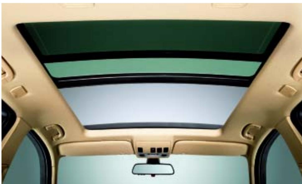
■ **Two-piece Panoramic moonroof** features fully electric slide and lift control. Both halves of the roof can be tilted up at the touch of a button. When you tilt the front glass section, the rear section also tilts up electronically. When open, the wind deflector minimizes turbulence. Includes comfort opening/closing function, and an electric sun shade to help shield cabin from excessive heat.
