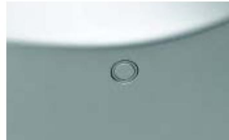
□ **Park Distance Control (PDC)**, front and rear, helps parking and maneuvering in tight spaces. The distance between your vehicle and an obstacle is indicated by an acoustic signal that increases in intensity as your bumper approaches the object, turning into a constant tone when the distance closes to 12 inches. A visual representation is also projected in the Control Display.
