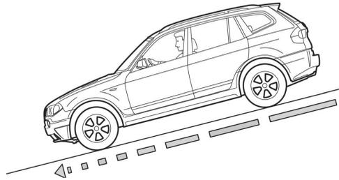
■ **Hill Descent Control (HDC)** helps the X3 drive down steep hills without having to “ride the brake.” By pressing the HDC button, the system keeps the X3’s speed under control automatically.
