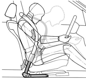
■ In the event of a severe frontal impact, **automatic safety belt tensioners** automatically tighten the lap and shoulder belts around front-seat occupants. **Always wear your safety belt and always place children in the rear seat.**
