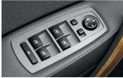
■ **Power windows** include "one-touch" up/down operation for the front and "one-touch" down for the rear.
