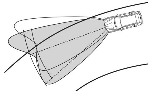
□ **Xenon Adaptive Headlights** automatically swivel to follow the curves of the road. The system uses data from on-board sensors and the steering wheel angle to determine the car's direction, then adjusts the headlights accordingly, for excellent nighttime vision.
