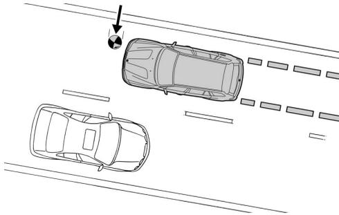
■ **Dynamic Brake Control (DBC)** senses “panic” braking maneuvers, and immediately builds up maximum brake pressure. This significantly cuts down the overall braking distance. When DBC is activated, the system also deploys **Adaptive Brake Lights**, warning following drivers brake quickly.
