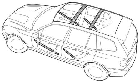
■ **BMW's door anchoring system** includes reinforcing bars with hook-like members within each door. In a serious side impact, the bars hook the door to the body, locking them together to make a more rigid passenger cell. When the pressure is released, the anchoring system is designed to disengage so that the doors can be opened (unless further damage from the impact prevents them from opening).
