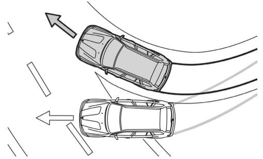
■ **Dynamic Stability Control** provides remarkable tenacity on slippery road surfaces. If the system senses over- or understeer, it modulates engine power and can apply brakes individually to help keep the vehicle under control and going in the intended direction.
