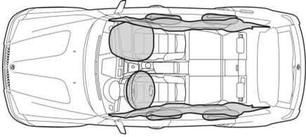
■ In the event of a collision, only the **airbags** that are needed are deployed. For the driver and front passenger, this includes “smart” front airbags, door-mounted side-impact airbags, and HPS (Head Protection System). For rear-seat passengers this includes HPS and optional rear side-impact airbags.
