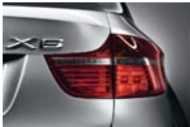
■ **Adaptive Brake Lights** increase vehicle visibility and signal the intensity of your braking action, thereby warning following drivers to brake quickly.
