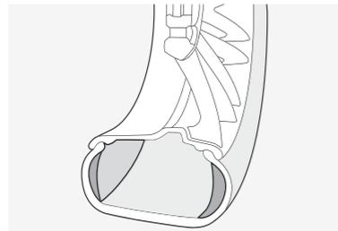
**Run-flat tires** allow speeds of up to 50 mph and travel from 30 to 150 miles after a loss of air pressure, depending on the passenger load and weight of articles being transported.<sup>1</sup> In situations that would normally result in a flat tire, reinforced sidewalls help prevent the tires from collapsing or loosening from the rim. In the event of a decline in tire pressure, the driver is warned by the **Tire Pressure Monitor**.
