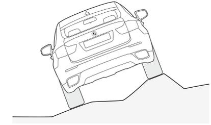
**Rollover sensor**, linked with the Dynamic Stability Control system, quickly detects when the X6 is at risk of rolling over and assists the driver in maintaining control of the vehicle. If a rollover is imminent, the airbags and the safety-belt pretensioners are immediately triggered to provide additional occupant protection.
