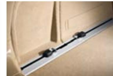
**Storage package** adds practical extras: additional lighting and two lashing rails with four sliding lashing eyes.
