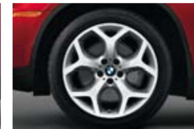
□ **Y Spoke (Style 214)** 20 x 10.0 front, 20 x 11.0 rear light alloy wheels with 275/40 front and 315/35 rear **run-flat<sup>1</sup> performance tires<sup>2</sup>** are available as an option when ordering the X6 xDrive35i Sport Package and Sport Activity Package. (Not available on X6 xDrive50i or ActiveHybrid X6.)
