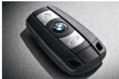
□ **Comfort Access system** offers an even greater degree of convenience: keyless access to your vehicle. Simply carrying the remote key in a pocket allows you to unlock the doors by touching the door handle. You can also turn the engine on or off by pressing the Start/Stop button without inserting the remote key. (Foot must be on brake in order to start.)
