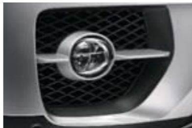
■ **Halogen free-form foglights** are cleanly integrated into the front air dam, illuminating the road ahead in bad weather and poor visibility. They also provide another practical feature: **Cornering Lights**. When the system senses you are making a turn ▮ based on your steering angle and speed ▮ a reflector mechanism in the foglight housing casts additional lighting up to 90 degrees in the direction of the turn. This enhances visibility and recognition of people and objects.
