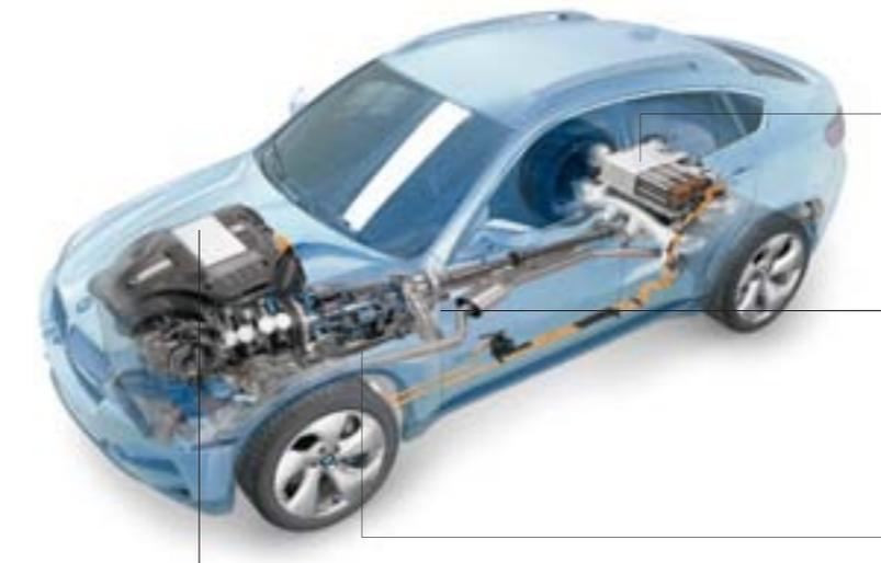
**Battery:** The high-performance nickel-metal hydride battery stored over the rear axle is powerful enough for daily use. Yet its compact design leaves ample room to stow four golf bags in the cargo area, as in the other X6 models.
