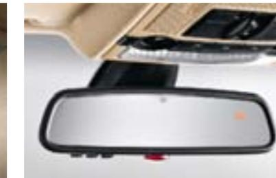
The **automatic-dimming inside rear-view mirror** darkens in response to the bright headlights of vehicles behind you. The easy-to-read **digital compass**, integrated into the mirror, is a convenient way to constantly keep your bearings while driving. A **three-button Universal garage-door opener** can be programmed to open garage doors and activate various remote convenience functions.
