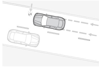
**Dynamic Brake Control** senses panic braking maneuvers, and immediately builds up maximum brake pressure. This cuts down the overall braking distance significantly. When Dynamic Brake Control is activated, the system also deploys **Adaptive Brake Lights**. These increase vehicle visibility and signal the intensity of your braking action, thereby warning following drivers to brake quickly.
