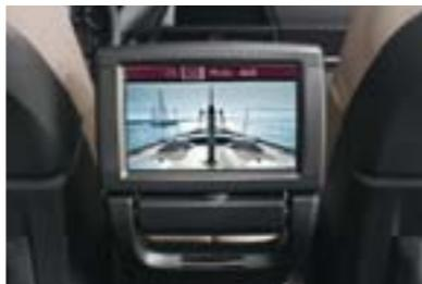
□ **Rear-seat entertainment** system lets passengers in the rear cabin watch DVDs or listen to their choice of CDs through headphones or the vehicle speaker system. The system features a fold-down 8-inch color screen and can be controlled via a wireless remote control or manually by the rear-seat passengers.
