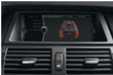
■ **Dynamic Performance Control Display** shows the percentage of drive force apportioned between the front and rear axles, as well as between the left and right rear wheels.
