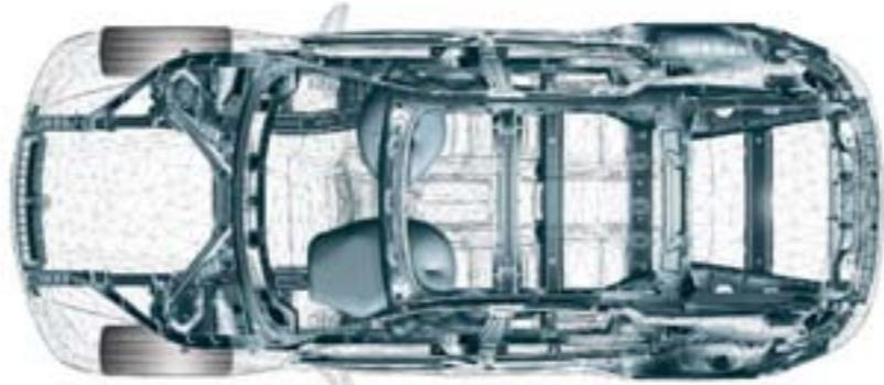
In the event of a severe impact, the X6's extremely rigid steel structure is designed to route impact forces around the passenger cell, and deform in a predetermined way. The **BMW Advanced Safety System** coordinates the activation of airbags, head restraints, safety-belt pretensioners and more, all helping to protect you and your passengers.
