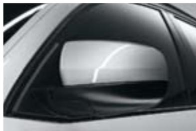
□ **Power-adjustable folding exterior side-view mirrors**, in matching body color, automatically dim when reflecting bright lights, helping to eliminate glare when driving at night. (Included in Premium Package.)
