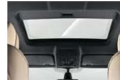
■ **Two-way power glass moonroof** with remote, expanded one-touch operation, slides back or tilts up to let in as much fresh air and sky as you like, while a wind deflector helps keep the wind out. Includes a sliding interior sunshade.
