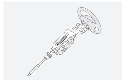
**Telescoping steering column system.** In a collision, a section absorbs a portion of the impact force and collapses, helping to protect the driver.
