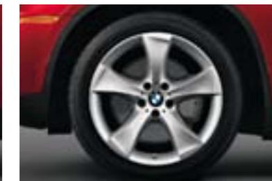
□ **Star Spoke (Style 259)** 20 x 10.0 front, 20 x 11.0 rear light alloy wheels with 275/40 front and 315/35 rear **run-flat<sup>1</sup> performance tires<sup>2</sup>** are available as an option when ordering the X6 xDrive50i Sport Package and Sport Activity Package. (Not available on X6 xDrive35i.)
