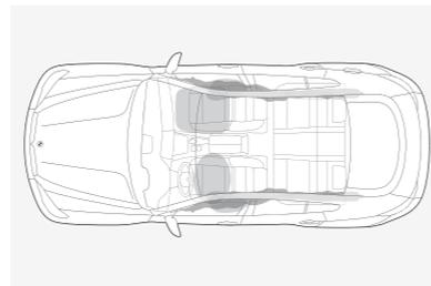
In the event of a collision, only the **airbags** that are needed are deployed. This includes front airbags with advanced deployment technology, front side-impact airbags, and front and rear HPS (Head Protection System).
