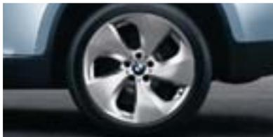
**Streamline (Style 297)** 20 x 10.0 front, 20 x 11.0 rear light alloy wheels with 275/40 front and 315/35 rear **run-flat performance tires**,<sup>1</sup> standard on the ActiveHybrid X6, reduce unsprung weight for increased performance.
