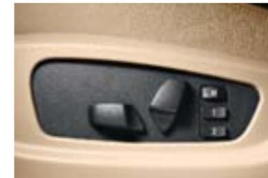
■ **Power seat adjustments** allow customized comfort for driver and front passenger. On the driver's side, a two-driver memory system automatically adjusts the driver's seat, side-view mirrors and the steering wheel position.
