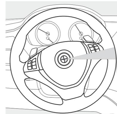
Greater agility at low and medium speeds: With Active Steering, a small turn of the steering wheel translates into a big turn of the front wheels.
