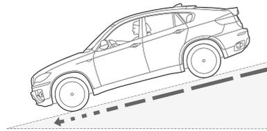
**Hill Descent Control (HDC)** helps the X6 drive down steep hills without having to ride the brake. By pressing the HDC button, the system keeps the X6's speed under control automatically.
