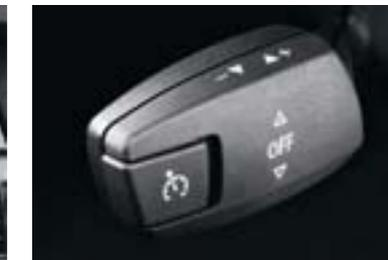
■ **Dynamic Cruise Control** lets you store and keep to a chosen speed above 20 mph, and automatically applies the brakes downhill. It is activated via the left-hand steering column switch, and deactivated by applying the brakes or via the switch.
