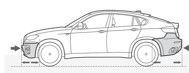
**Impact-absorbing bumpers** and compressible crush tubes front and rear help absorb the force of impact in collisions up to nine mph, minimizing damage to the vehicle's body and simplifying repairs. Only at higher impact speeds do structural supports begin to deform, dissipating impact energy to help protect occupants.
