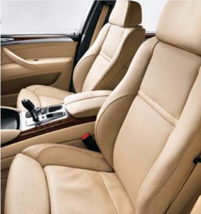
**20-way power multi-contour front seats** conform to your body to provide optimum support and exceptional comfort over long distances. In addition to horizontal, vertical and angled adjustments, multi-contour seats include an articulated upper backrest, backrest width, Comfort headrest (two-way power, two-way manual "relax headrest"), and four-way power-adjustable lumbar support. Both driver's and front-passenger's seats include memory function.
