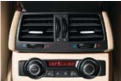
**Four-zone climate control** lets occupants, both front and rear, select individual temperature and fan settings.
