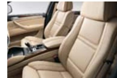
■/□ **20-way power multi-contour front seats** conform to your body to provide optimum support and exceptional comfort over long distances. In addition to horizontal, vertical and angled adjustments, seats include an articulated upper backrest, backrest width, Comfort headrest (two-way power, two-way manual || relax headrest!), and four-way power-adjustable lumbar support. Both driver's and front-passenger's seats include memory function.
