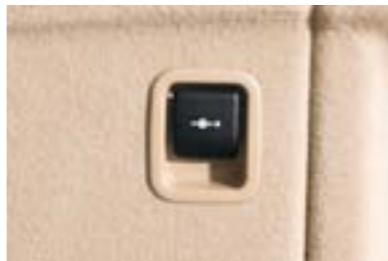
■ **12V power outlets** are included in the front and rear passenger areas, as well as in the cargo area.
