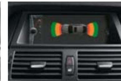
■ **Park Distance Control** uses eight sensors **four** in the front, **four** in the rear **to** help you judge how close you are to other cars and unseen objects when parking. The warning beeps come faster as the bumper approaches the object, turning into a constant tone when the distance is less than 12 inches.
