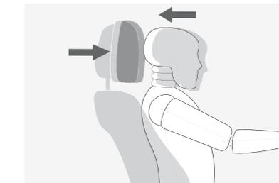
**Active Head Restraints** in the front seats reduce the risk of whiplash or neck/head/spine injury. When sensors detect a rear-end collision, the headrests rapidly and automatically pivot forward, supporting the driver's and front-seat occupant's heads.
