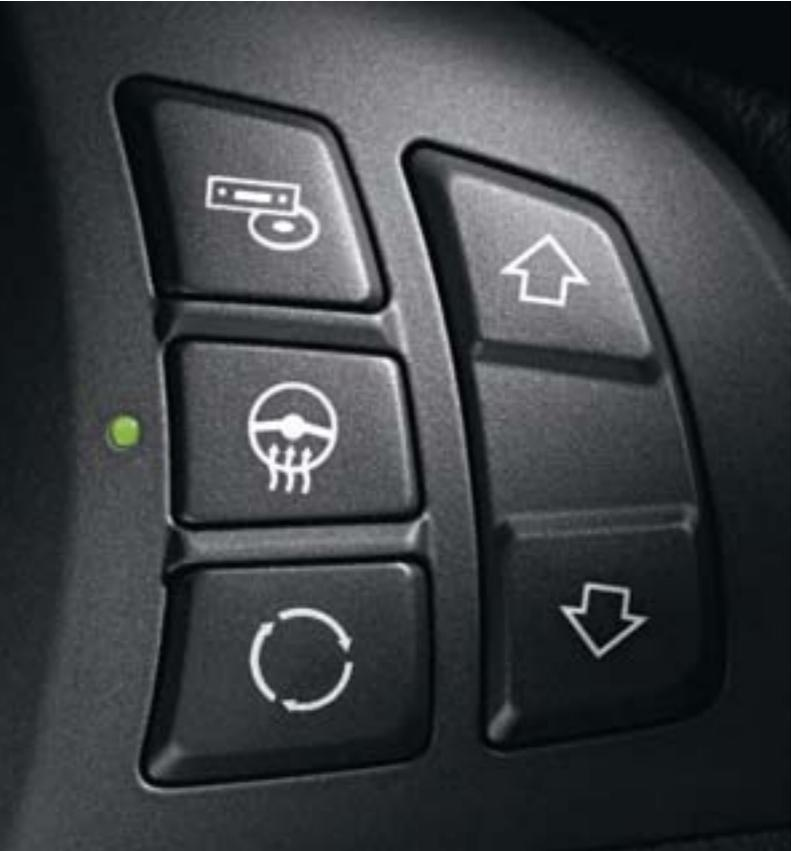
**Heated steering wheel** is a feature that, like heated seats, becomes a "must-have" once it's experienced. The heating switch is conveniently located on the multi-function steering wheel.
