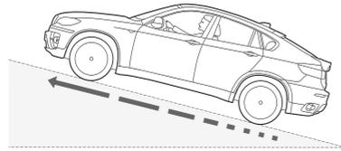
**Start-off Assistant** keeps the X6 from rolling either backward or forward when you're stopped on a hill. The system momentarily holds the X6's position as you take your foot off the brake pedal and start driving.
