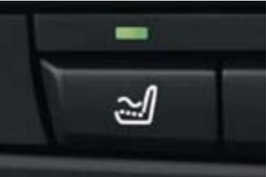
**Active driver's seat** helps decrease stiffness or fatigue on long trips. When activated, the driver's seat surface is continuously and imperceptibly raised and lowered from side to side, keeping your spine in motion and exercising various support muscles.
