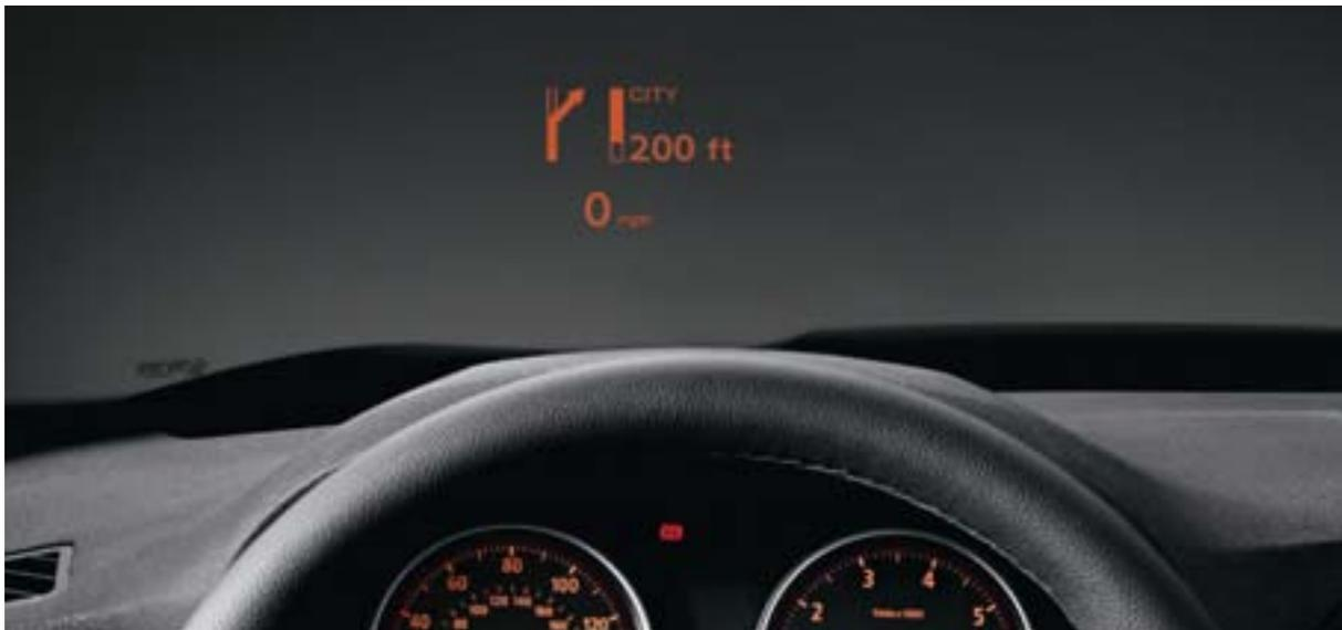
□ **Head-up Display** projects important travel information, such as current speed, on the windshield directly in the driver's line of vision. Directional arrows from the Navigation system and Check Control data can also be displayed.
