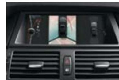
□ **Rear-view camera with Top View** is activated automatically by shifting into reverse gear, or manually by pressing the parking-assist button. The color display shows a real camera image that may include **static** and **track** lines to help you when backing up or parallel parking.
