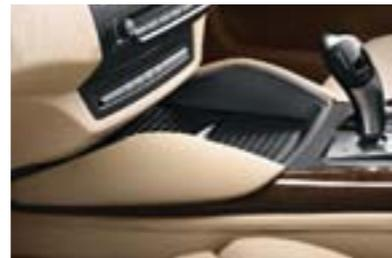
■ **Kneepads** along the sides of the center console provide greater comfort and grip for the driver and front passenger's knees || especially during quick, sharp turns.
