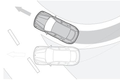
**Dynamic Stability Control** provides remarkable tenacity on slippery road surfaces. If the system senses over- or understeer, it modulates engine power and can apply brakes individually to help keep the vehicle under control and going in the intended direction.
