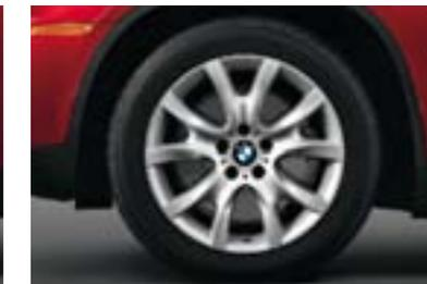
■/□ **V Spoke (Style 257)** 19 x 9.0 light alloy wheels with 255/50 **run-flat<sup>1</sup> all-season tires** are standard on the X6 xDrive50i and optional on the ActiveHybrid X6.
