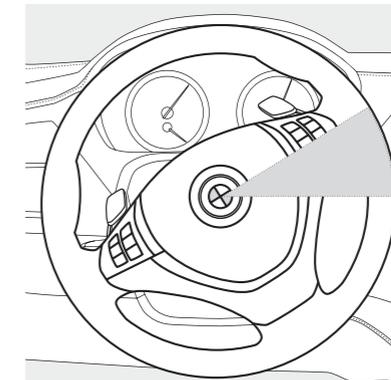
At higher speeds, greater stability and precision: A bigger turn of the steering wheel is needed to turn the front wheels.
