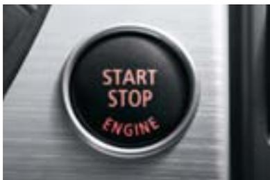
■ **Engine Start/Stop button and remote key** control the engine. First, insert the remote key into the starter switch slot. After the electronic identification system confirms that it is the correct remote key, you can start (or later, turn off) the engine by pressing the Start/Stop button. (Foot must be on brake in order to start.)
