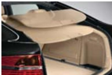
■ **Retractable cargo cover** keeps contents of the cargo area hidden from sight. When not in use, it can easily be removed.
