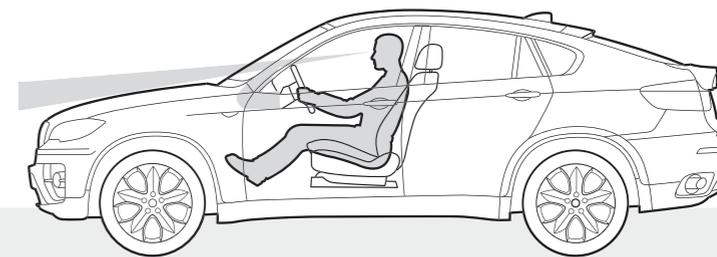
**The Head-up Display shows relevant information, such as the car's speed, directly into the driver's field of vision. The height-adjustable display helps keep you focused on what's happening on the road.**
