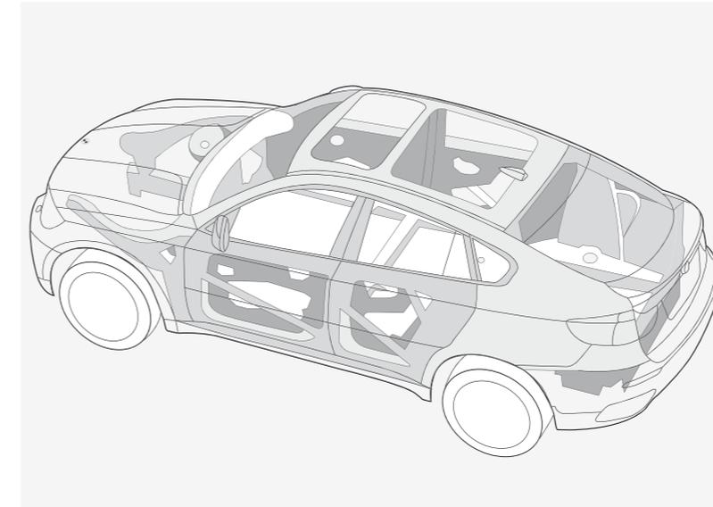
**Extremely rigid body** creates a protective safety cell that directs severe impact forces around the passenger compartment. Thanks to BMW's intelligent lightweight design and the use of high-strength steels, the interior passenger compartment is surrounded by a stronger shell than was previously possible to construct.
