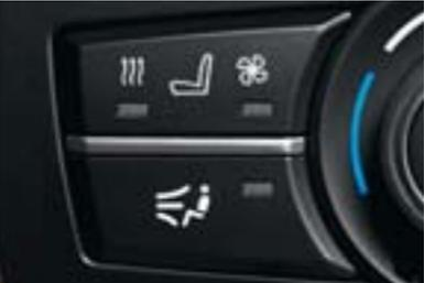
**Front seat ventilation** gently blows warm air or cool air through the microperforations in the leather to help keep driver and front passenger comfortably dry in hot weather, and warm in colder weather.
