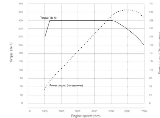
**Portrait of an engineering masterpiece: the X6 xDrive35i Advanced Turbo engine produces 300 hp at 5800 rpm, and quickly develops 300 lb-ft of torque at 1400 rpm, which continues without fading through to the 5000 rpm range. With such a broad range of powerful torque, you can enjoy smooth, robust acceleration in any gear, at any speed.**
