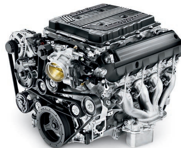
6.2L LT4 SUPERCHARGED V8 (STANDARD ON Z06)
