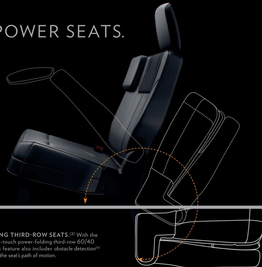
**EXCLUSIVE ONE-TOUCH POWER-FOLDING THIRD-ROW SEATS.<sup>(2)</sup>** With the touch of a button the available class-exclusive one-touch power-folding third-row 60/40 split-bench seat<sup>(2)</sup> folds directly into the floor. This feature also includes obstacle detection<sup>(4)</sup> to automatically pause if something is detected within the seat's path of motion.
