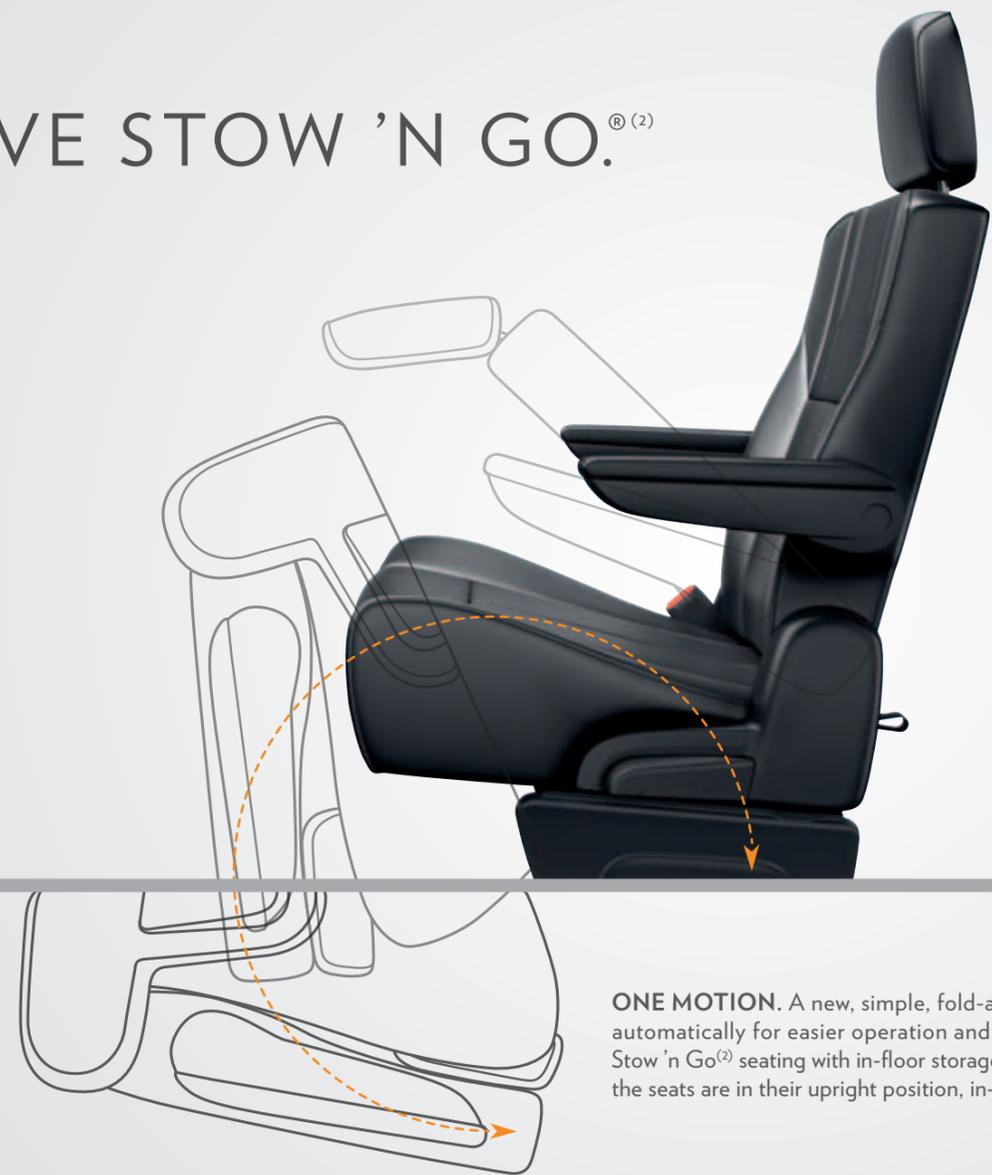
**ONE MOTION.** A new, simple, fold-and-stow system now allows the head restraint to fold down automatically for easier operation and reveals what makes Town & Country legendary: exclusive Stow 'n Go<sup>(2)</sup> seating with in-floor storage bins and fold-in-floor second- and third-row seats. When the seats are in their upright position, in-floor bins are available to accommodate carry-ons.
