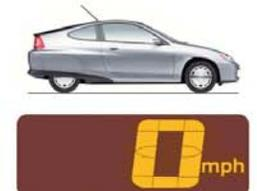
**At a stop** the engine cuts off to reduce fuel consumption and emissions, thanks to the automatic **idle-stop feature**. And when you're ready to go again, it starts up by itself.
