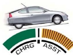
**Acceleration** is strong and responsive, as the **IMA motor** augments the output of the **gasoline engine**. The IMA assist indicator lights to show current flow from the batteries.
