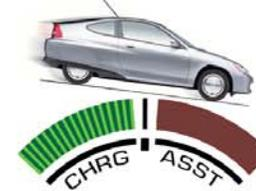
**Braking** is regenerative for the IMA motor's battery pack, tapping into the Insight's kinetic energy. Here, the IMA electric motor automatically becomes a highly effective **generator**.
