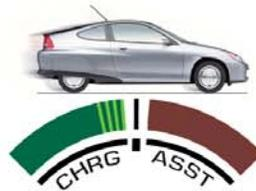
**Cruising** at a steady speed puts the Insight's low-emission, fuel-efficient<sup>2</sup> **1.0-liter VTEC-E** engine to work by itself. And as the charge indicator shows, the batteries receive some current.
