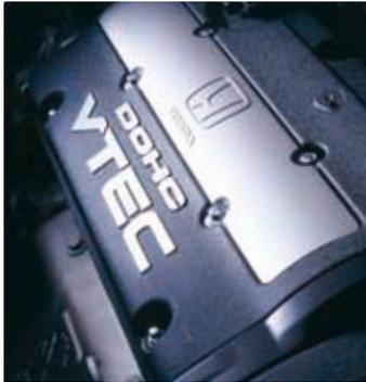
A 200-hp, 2.2 liter, 16-valve, DOHC VTEC 4-cylinder engine gives the Prelude its high-revving power. Dual overhead camshafts allow the valves to be more optimally placed, resulting in increased power.
