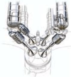
Honda's patented VTEC variable valve-timing system smoothly switches between low- and high-lift camshaft profiles that better match air/fuel flow with engine demands from low to high rpm.
