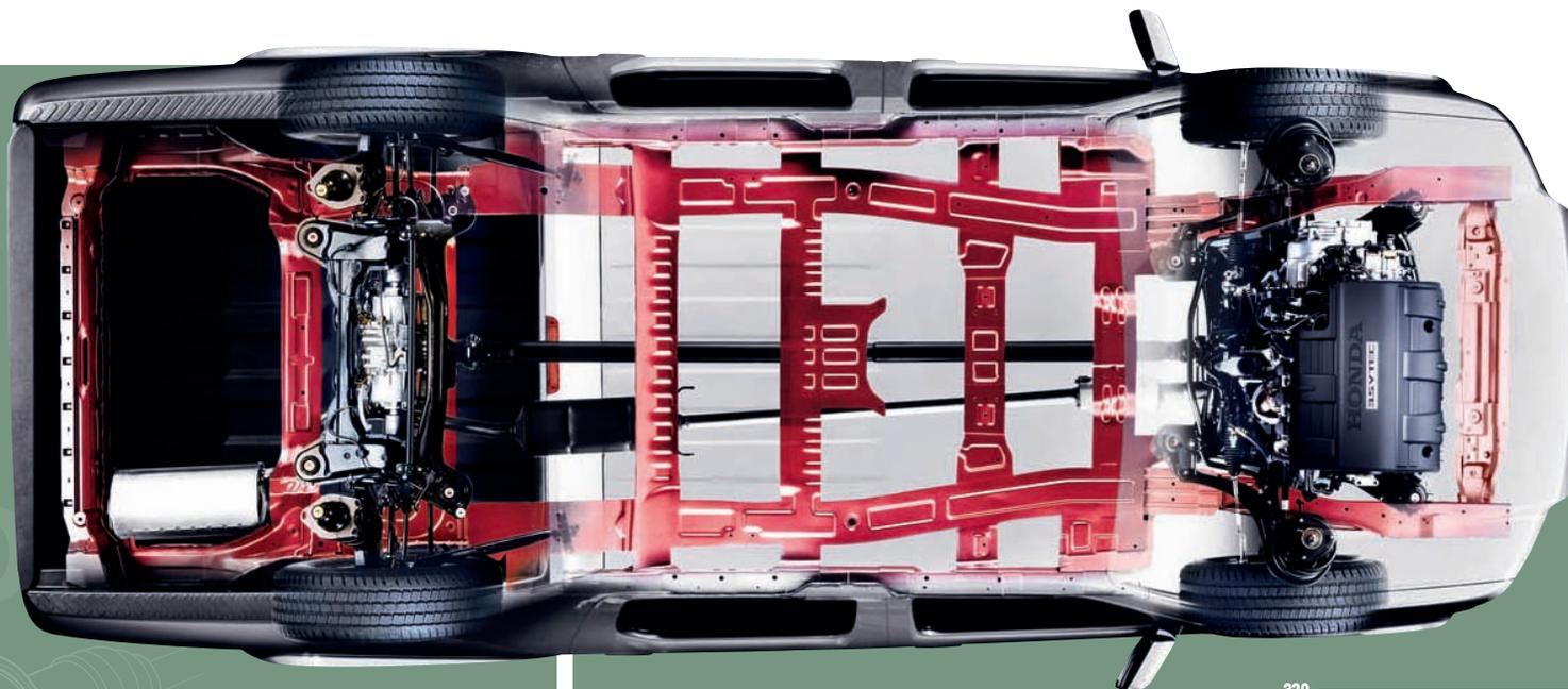
Like most 4-wheel-drive systems, the Ridgeline responds reactively to wheel slippage, sending power where it's needed most. But unlike competing systems, it also responds proactively based on the amount of torque the engine is producing. By anticipating the need to send power to additional traction points, it ensures a smooth and almost transparent transition between 2- and 4-wheel drive.
