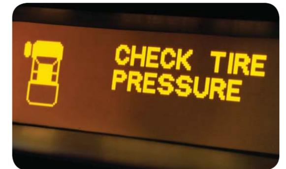
The Ridgeline's standard Tire Pressure Monitoring System (TPMS)§ continually checks the pressure of each tire, alerting the driver with an in-dash display when a particular tire's pressure is significantly low.
