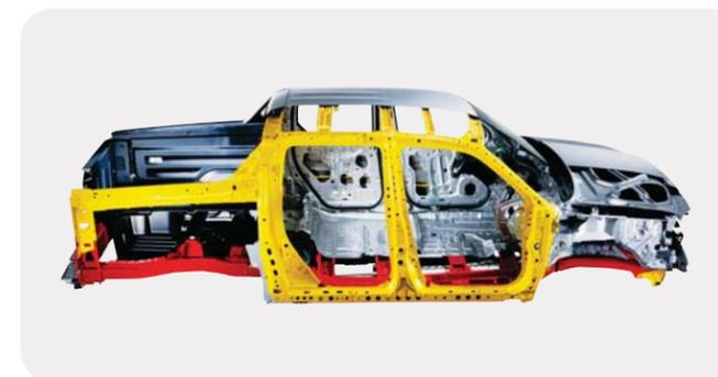
The Ridgeline's first line of defense is a reinforced unit body that incorporates a closed-box frame with internal high-strength steel frame stiffeners. Both the frame rails and all seven crossmembers feature box-section construction. The result is a remarkably high torsional rigidity.
