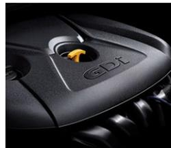
**ENGINE INNOVATIONS** Elantra Sport's new engine is an all-aluminum design whose light weight aids in fuel efficiency. To help ensure durability, our engineers designed the D-CVVT valve train to be driven by a long-lasting steel chain (instead of rubber belts) and specified hydraulic motor mounts to minimize vibration in the chassis.
