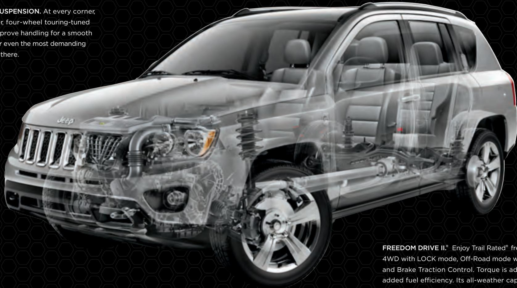
**FREEDOM DRIVE II.<sup>®</sup>** Enjoy Trail Rated<sup>®</sup> freedom, thanks to full-time 4WD with LOCK mode, Off-Road mode with Hill Descent Control, and Brake Traction Control. Torque is adjusted on-demand for added fuel efficiency. Its all-weather capability expertly handles more difficult off-road situations, as well as deeper snow, mud, and up to 19 inches of water.<sup>2</sup> Available.
