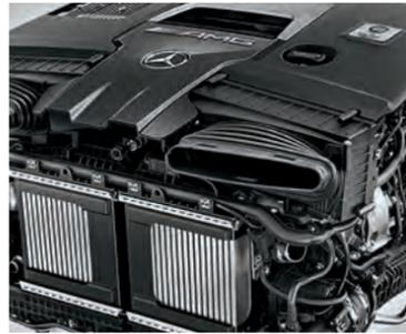
AMG-enhanced turbo inline-6 with EQ Boost Integrated Starter-Generator (ISG), or handcrafted AMG biturbo V8
