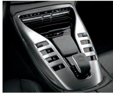
V-shaped console with color display buttons and capacitive switches
