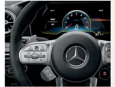
Touch Control Buttons on steering wheel, touchpad on console
