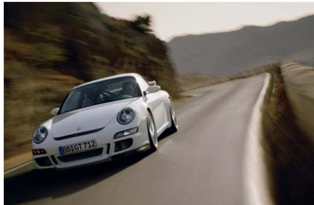
The one-piece 19-inch GT3 wheel features lightweight construction and a road-approved sport tyre (see page 53). The special tread and compound enable higher cornering speeds as well as precision handling and turn-in characteristics.
