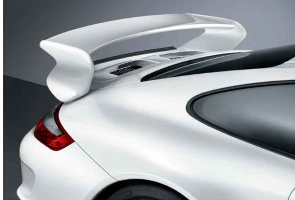
The most prominent feature at the rear of the car is the fixed bi-plane wing structure. The angle of incidence on the upper wing element can be adjusted for racing use. It also offers even greater stability at high speed. An interesting detail on the lower wing surface is the smaller rubber spoiler or 'Gurney flap'. This device creates additional downforce with a negligible increase in drag.
