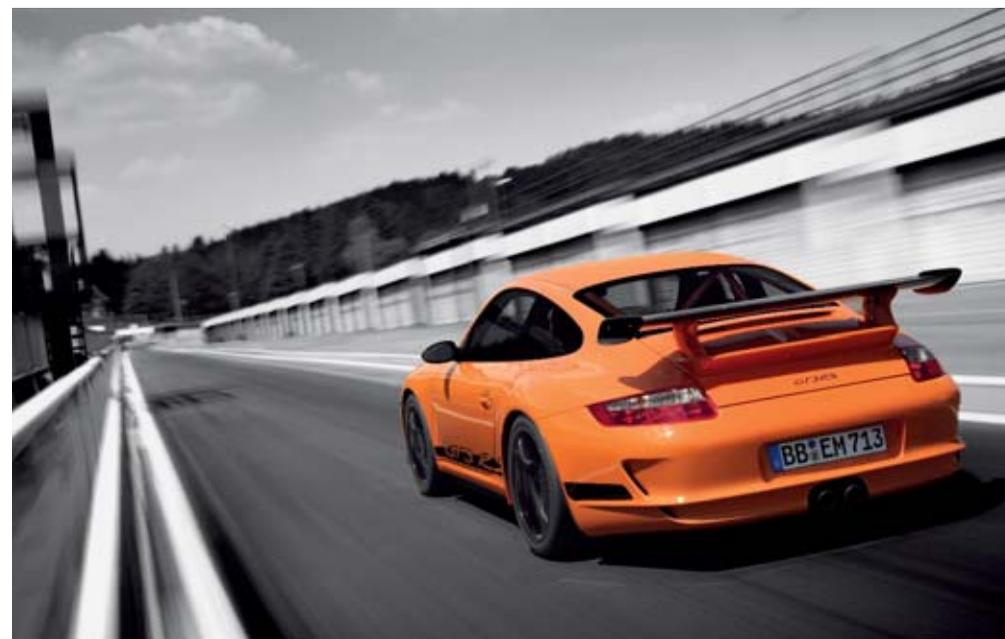
Another feature shared with the 911 GT3 are the lightweight 19-inch GT3 alloy wheels. The rear rims have a smaller offset, accommodating a 34-mm increase in track. This additional width helps to minimise roll when cornering. The wheels are fitted with road-approved sport tyres offering excellent traction and grip.
