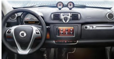
**Additional instruments:** both cockpit clock and rev counter are illuminated from the inside and swivel easily to align perfectly with driver's field of vision. Available on passion models.
