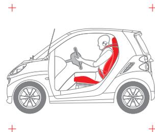
**Safety seats with integrated seat belts and belt tensioners:** the sheet steel structure with integrated headrests provides the smart fortwo's seats with a high level of mechanical stability. In a frontal impact, the seat belt tensioner reduces slack within milliseconds. The belt-force limiter then reduces the force again to minimize pressure on the driver and passenger.
