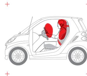
**Full-size airbags and head/thorax side airbags:** in a frontal impact, two full-size front airbags provide maximum protection for driver and passenger. In the event of a side-on impact, the doors' robust steel structure and head/thorax side airbags afford additional protection for the head and chest. Standard on passion cabriolet. Coupe models have 2-side and 2 window airbags. Driver and passenger knee bolster airbags come standard on all models.
