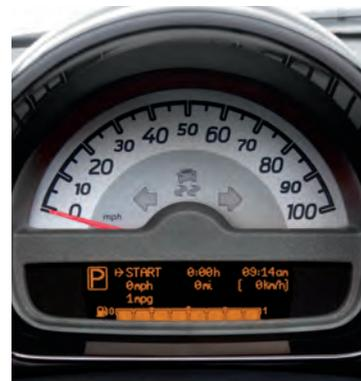
**Trip computer:** the easy-to-read multi-functional display shows current fuel consumption, mileage, trip information and more. Operated via the steering column control stalk. Available with cruise control package.
