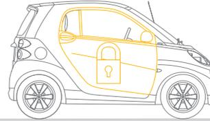
**Drive lock function:** this locks the doors automatically once the vehicle reaches approximately 8 mph.
