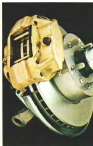
*The Volvo 164E has 4-wheel self-adjusting power disc brakes and two separate braking systems. Each operates on the two front wheels and one rear wheel. Since each front brake*
