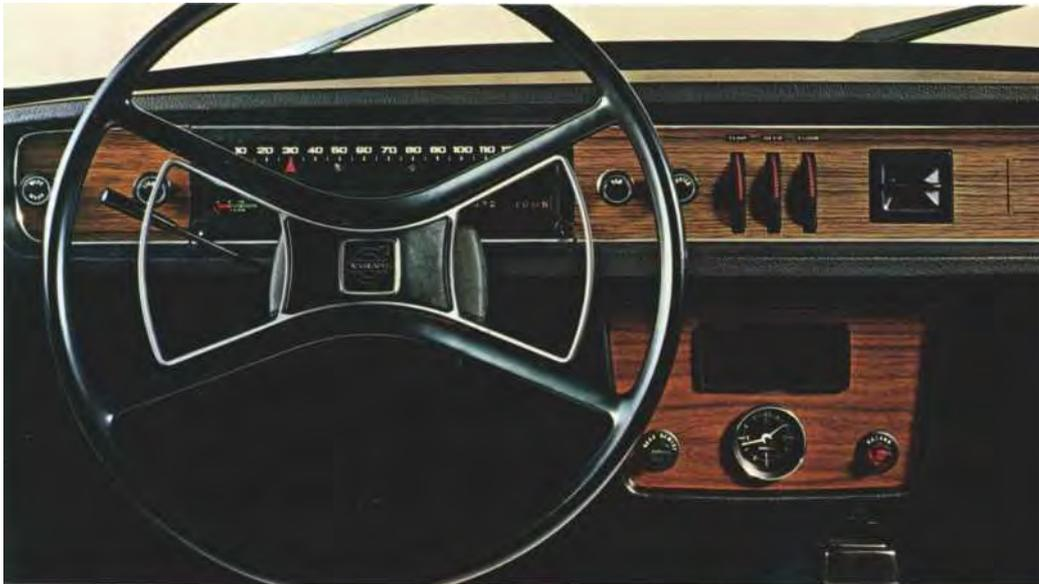
*A new center console contains the electric clock with plenty of room left over for the air conditioning you may wish to add.*
