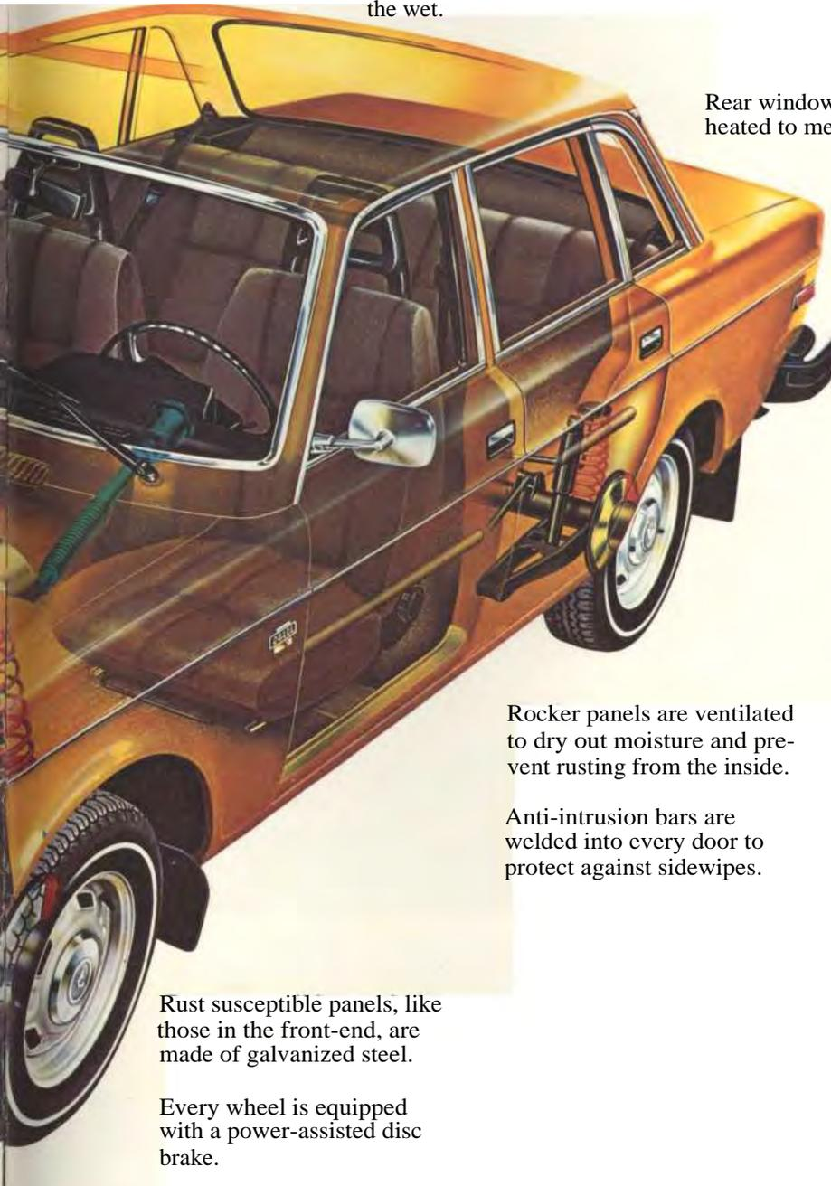
Rear window is electrically heated to melt ice.
