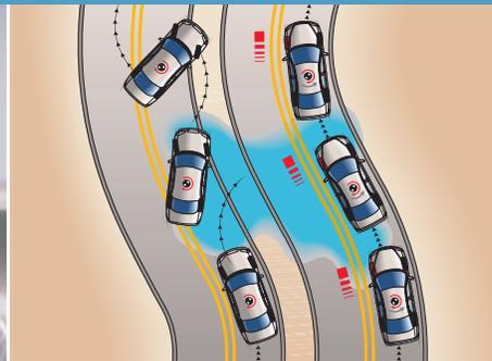
**DSC ANTI-SKID SYSTEM (DYNAMIC STABILITY AND TRACTION CONTROL)**
