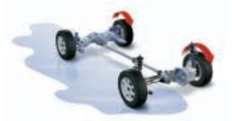
If one or both wheels on one side of the car spin, more power goes instantly to the wheels on the opposite side with the best traction.
