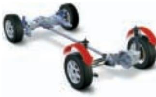
When braking, the car disengages drive to the rear wheels the instant you touch the brake pedal, thereby maximizing control and roadholding.
