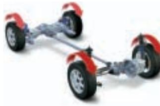
If the front wheels show any tendency to spin, the AWD system responds instantly by redistributing up to 50% of the power to the rear wheels for maximum traction and stability.
