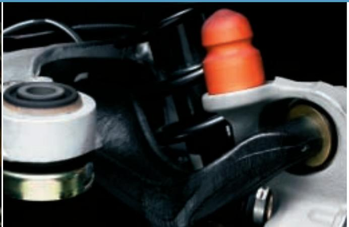
The sophisticated multi-link rear suspension contributes to the excellent riding comfort and ensures well-balanced behavior on the road. Its design also enhances the car's supple steering characteristics – in a curve, the rear wheels steer slightly in the same direction as the front wheels for added stability.
