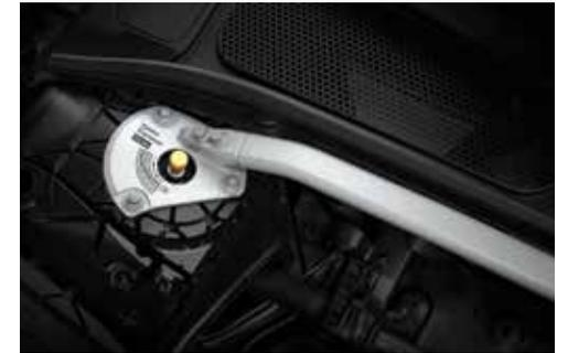
The front suspension is further stabilized by a Polestar Engineered strut bar. This contributes to even more precise, responsive steering characteristics at all speeds and more controlled handling through the curves.
