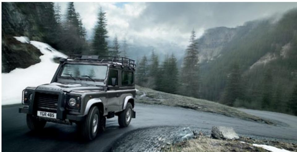
Vehicle shown right is accessorised with Expedition Roof Rack System, Two Part Rear Access Ladder, Raised Air Intake, Wing Top Protectors, Front Lamp Guards, A-Frame Protection Bar, Ribbed Aluminium Undershield, Front Mudflaps, 16 inch 5-Spoke Alloy Wheels - Dual Finish and Folding Side Step.
