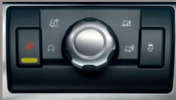
**TERRAIN RESPONSE®** Land Rover's patented Terrain Response® system adds to Land Rover LR2's breadth of capability. Any of the four settings – general driving, grass/gravel/snow, mud and ruts, or sand – can be easily selected by simply turning the rotary control. In addition all vehicles with Terrain Response® are also fitted with Hill Descent Control and Land Rover's Gradient Release Control systems.
