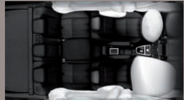
**SAFETY** Ultra-high-strength steel is used to construct an immensely strong monocoque body and inner safety cell protected by front and rear energy absorbent crumple zones. Seven airbags are fitted as standard on all vehicles.
