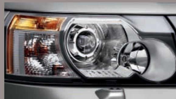
**HEADLIGHTS** Standard halogen headlights with impact-resistant polycarbonate lenses. Optional Adaptive Xenon projector lamps providing crisp blue-white light letting you see further and automatically swivel with the direction of travel to improve the view of the road ahead.
