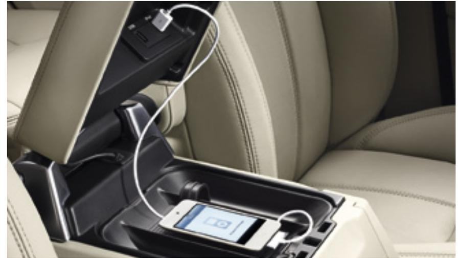
**THE PORTABLE AUDIO INTERFACE.** Allows the connection to the in-car entertainment system of an iPod® with full track and search integration. An MP3 player or a mass storage device can also be connected via the USB port. Bluetooth® audio streaming is also available enabling music to be played through the in-car entertainment system via a Bluetooth® connection.
