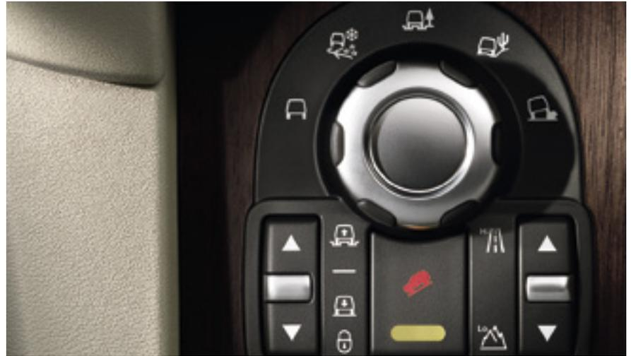
**TERRAIN RESPONSE® SYSTEM†.** Standard on every Land Rover LR4 and optimizes the vehicle set-up for virtually all on-road or off-road driving situations, with five different settings to suit different terrains such as Grass/Gravel/Snow, Sand, Mud and Ruts and Rock Crawl.
