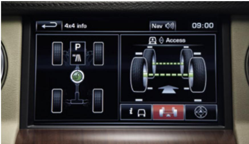
**AIR SUSPENSION.** Standard four-corner independent air suspension features variable ride height and electronic cross-linking for a constant level ride height irrespective of passenger load distribution. Ride height can be raised up to 2.2 inches/125mm to clear obstacles or lowered by 1.9 inches/50mm for easy access and loading.
