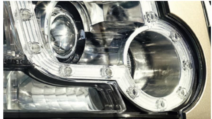
**AUTOMATIC HEADLAMPS WITH HIGH BEAM ASSIST\*.** Detect vehicle headlamps/tail lights and dip the high beam until the light source is out of range. The system is able to distinguish between automotive and non-automotive light sources.
