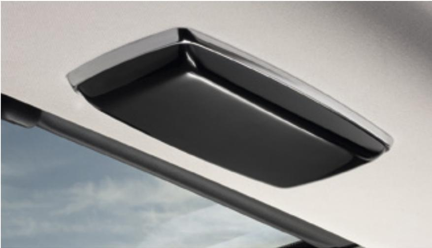
**WHITEFIRE®.** This technology is a wireless system, discreetly housed in a unit in the vehicle's headlining, which allows the convenient use of cordless headphones with the optional rear seat entertainment system.
