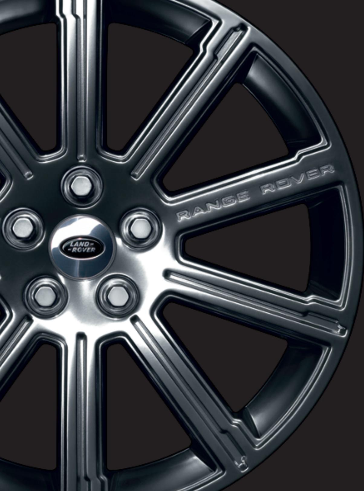
The new 2010 Range Rover's alloy wheels are manufactured from extremely resilient material. They are designed to enhance the vehicle's appearance as well as improve handling by reducing unsprung weight, allowing the suspension to react more quickly. Not only has each one been through a series of formidable tests, to simulate on-off-road stresses, every individual wheel is also x-ray checked by the wheel manufacturer.
