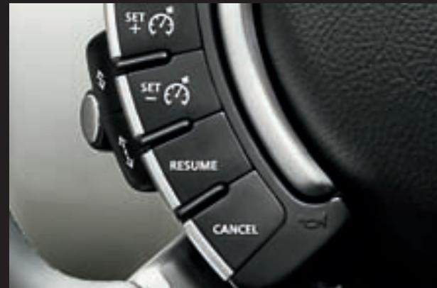
The Adaptive Cruise Control System can be programmed to one of four settings of between a 1.0 second and 2.2 seconds interval from the vehicle in front in normal driving conditions or when Grass, Gravel, Snow is selected on the Terrain Response® dial.
