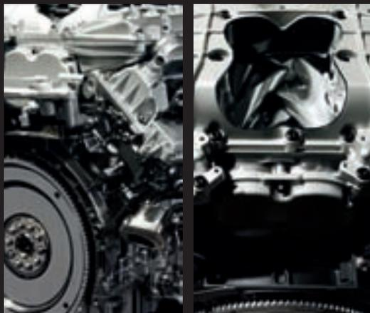
The new LR-V8 Engines feature 'drive by wire' throttle control and camshaft profile switching to increase torque and improve performance.
