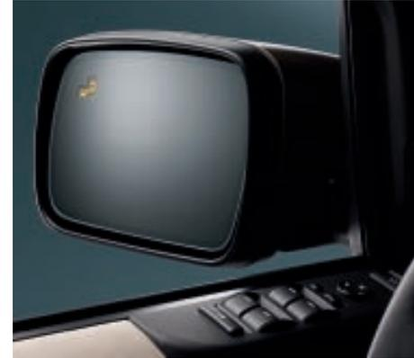
Side-mounted radar gives the available Blind Spot Monitoring system the ability to warn of vehicles that the driver may not see. A bright amber warning icon is illuminated in the appropriate door mirror when a hazard is detected.
