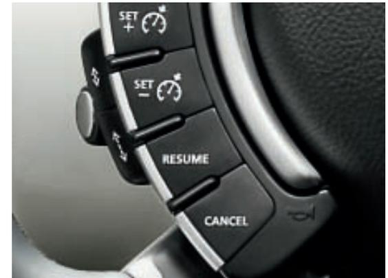
Available Adaptive Cruise Control has four driver-selectable settings, designed to suit individual driving styles and traffic/road conditions.
