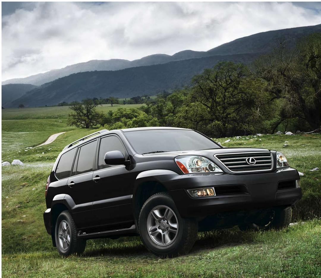
The GX is equipped with a 4.7-liter V8 engine, unleashing 263 horsepower<sup>2</sup> and 323 lb-ft of torque.<sup>2</sup> Taming this beast is Variable Valve Timing with intelligence (VVT-i), which continually monitors and adjusts the engine's valves to deliver optimum performance at all times. And a five-speed Electronically Controlled Transmission (ECT) keeps everything running smoothly.
