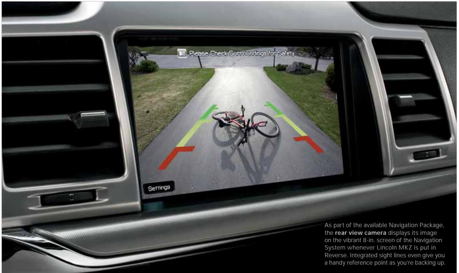
As part of the available Navigation Package, the **rear view camera** displays its image on the vibrant 8-in. screen of the Navigation System whenever Lincoln MKZ is put in Reverse. Integrated sight lines even give you a handy reference point as you're backing up.
